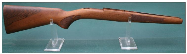
butt plate with Musgraves logo on it. There was some minor transit marks but no major damage and no signs of weakness to the design. The stock was fitted with the old style sling swivels and I will as part of the restoration process replace this with Uncle Mikes QD swivels. Restoration of the stock was simplicity itself and consisted of removing the old finish, removing the transit marks, creating a suitable final surface and applying a matt oil.
