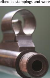
To protect the muzzle thread I have fitted a thread protector.
