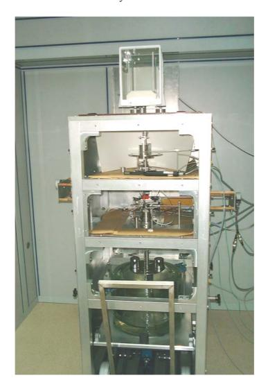
A view of the hydrostatic weighing device is shown in the photo. At the top is a commercial mass comparator. Suspended from the balance pan are two auxiliary pans, connected in series. One of these (seen in the upper chamber) is used for weighings in air and the second (seen in the lower chamber) is used for weighings in water. In the photo, two cylindrical mass standards have been loaded onto a weight
