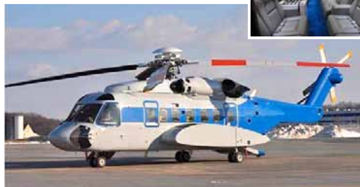
▲ The standard S-92 aircraft includes a spacious cockpit with excellent exterior visibility, a stand-up cabin for up to 19 passengers, modern avionics with large NVG-compatible displays, a crashworthy fuel system separated from the passenger compartment, and a rear ramp for loading passengers or cargo.
