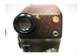
When the camera is switched over to sync 24 fps the red light above and to the right of the sync switch will flicker brightly and constantly. When the camera is shooting at variable speeds the light will fade in and out and the flickering of the light will not look constant. This light can also be a warning if the camera is out of sync. If the light fades in and out even in sync 24 than the camera is not in sync.
