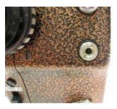
Located to right (right-rear) of the viewfinder, this socket takes a special electronic remote control lead plug, which is included in all rental packages. You must use this remote release cable in the socket for any frame rate above 24, (slow-motion).
