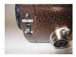
The crystal speed module is located below the eyepiece. It will govern the camera's running speed assuring a constant speed, allowing sound to be recorded on a separate sound recorder. You may switch to variable speeds: 2 - 70 fps or sync 24 fps.
