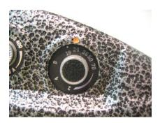
This dial makes it possible to set the camera at the desired filming speed between 2 and 70 fps. If your *Classic Camera* is equipped with a power lens, the camera will automatically correct the diaphragm for proper exposure according to the shutter speed selected. This makes it possible to change run speeds during filming. (It is also possible to change filming speeds with a "manual" lens, but the exposure will have to be calculated separately.)
