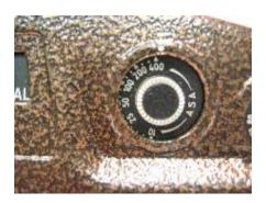
This dial allows you to select the ASA/ISO setting for the internal exposure meter. *Note: The 400 ASA setting should be used for 500 ASA films*.
