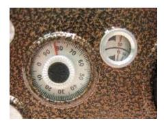
This indicates the footage still available, both in frames and in feet. The counter automatically resets to zero when the film is unloaded.
