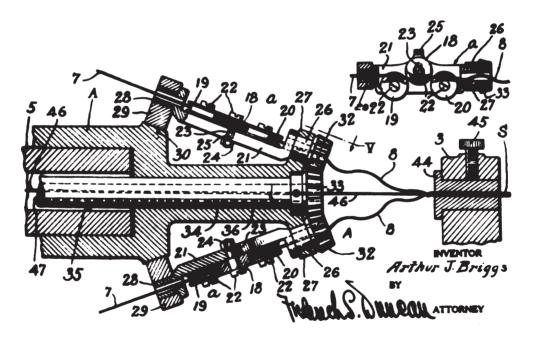
Fig. 17: Briggs' preforming head with rollers
