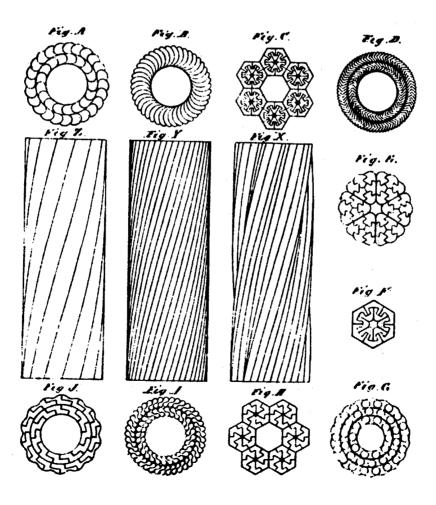
Fig. 18: Latch & Batchelor's locked coil ropes
