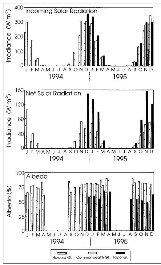
Figure 1. Mean monthly incoming solar radiation (top panel), net solar radiation (middle panel), and albedo (lower panel) of three glaciers in Taylor Valley, Antarctica, during 1994–1995. Measurements did not begin on Taylor Glacier until 1995. Data are missing from the Commonwealth Glacier in October 1994 due to data-logger failure. Albedos are calculated only for time periods in which light is present.
