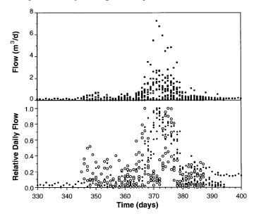
Figure 1. Daily discharge values in 1993–1994 and 1994–1995 austral summers for eight streams in the Lake Fryxell basin, Taylor Valley, Antarctica. (*Top*) Discharge values in cubic feet per day. (*Bottom*) Daily discharge as a fraction of maximum discharge per stream for each year. Filled circles: 1993–1994; open circles: 1994–1995. (cf/d denotes cubic feet per day. Multiply cubic feet by 0.03 to obtain cubic meters.)
