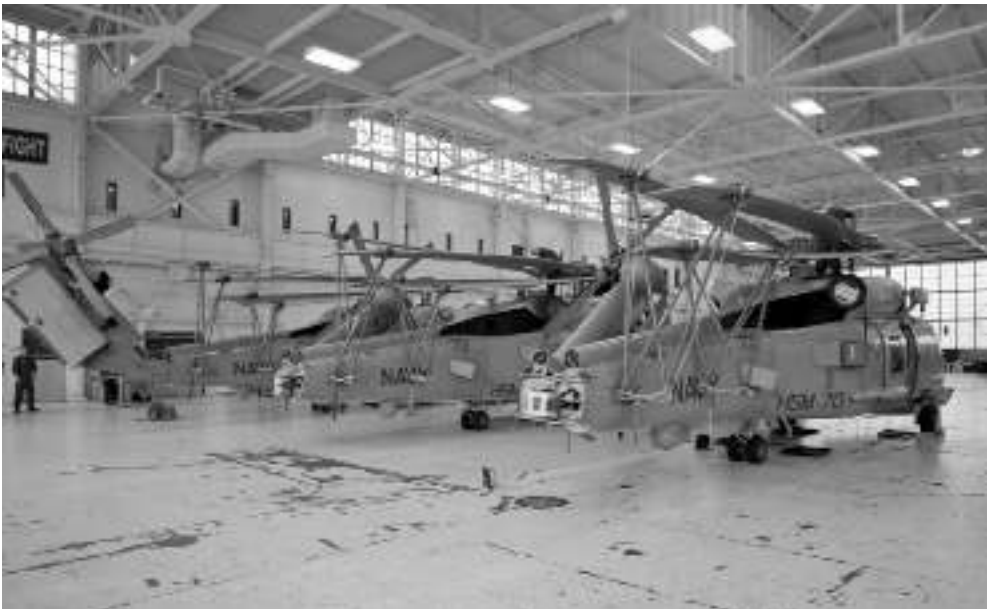
Three of the four new delivered MH-60R helicopters of HSM-70 are visible here. Clearly visible under the fuselage is the FLIR pod. These MH-60Rs also show the folding tail and folded stabilo to reduce space when hangared.
