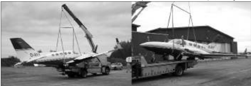
As can be seen in these pictures by Jack Poelstra, Cessna Golden Eagle II IIYY received only minor damage when upon landing at Groningen-Eelde the left main gear collapsed, sending the twin prop into the grass with two students of the Dutch Flight Academy on board. As soon as the gear is back in its normal position and the grass is cut from the left engine cowling and flaps, it should be in the air before long.
