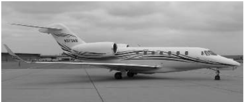
Winglets remain hot in this period where fuel savings are becoming more and more important, both to manage the economic crisis and global warming. The latest aircraft to have these drag reducing features is the Cessna 750 Citation X. The first customer aircraft with elliptical winglets we know of is this N373AB of Salem Aviation. Oliver Schmid photographed the bizjet at Stuttgart on 15 September 2009.
