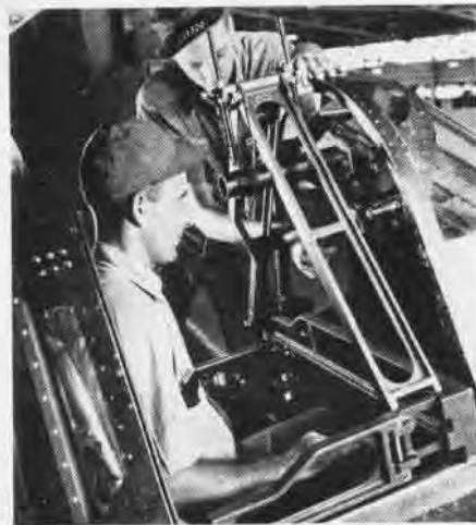
BORESIGHT FIXTURE INSTALLED IN SB2C
