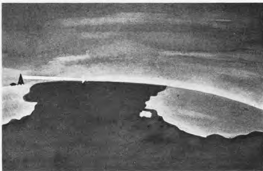
RANGE OF LORAN TRANSMITTERS IS GREATER AT NIGHT THAN DAY DUE TO SKY WAVES
