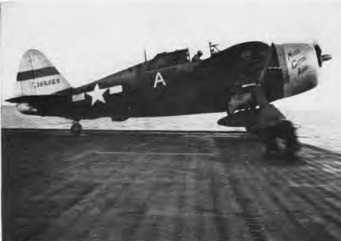
Natoma Bay catapults Army P-47 to bolster Saipan offense; these escort carriers, thanks to catapults, can carry whole deck load of planes
