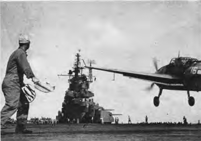
Yielding elements hold arresting gear wire off deck of Yorktown so that Avenger's hook will catch it. The LSO has given pilot the cut
