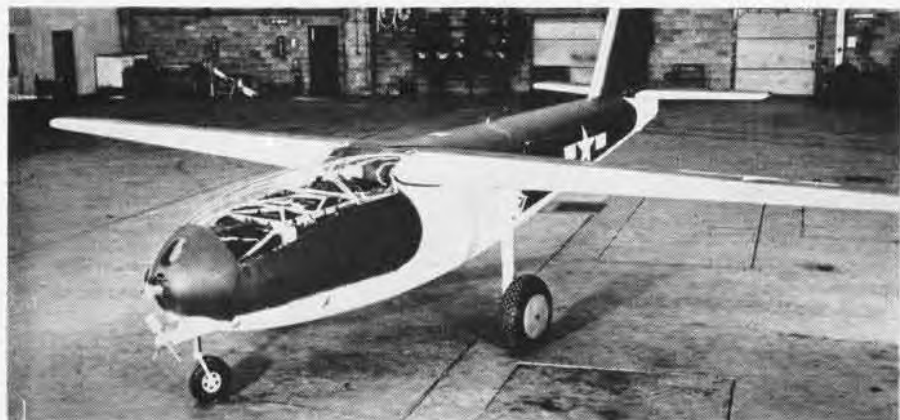
HIGH WING PIPER MONOPLANE, ONE OF 'GLOMB' FAMILY, CARRIES A 4000-POUND BOMB
