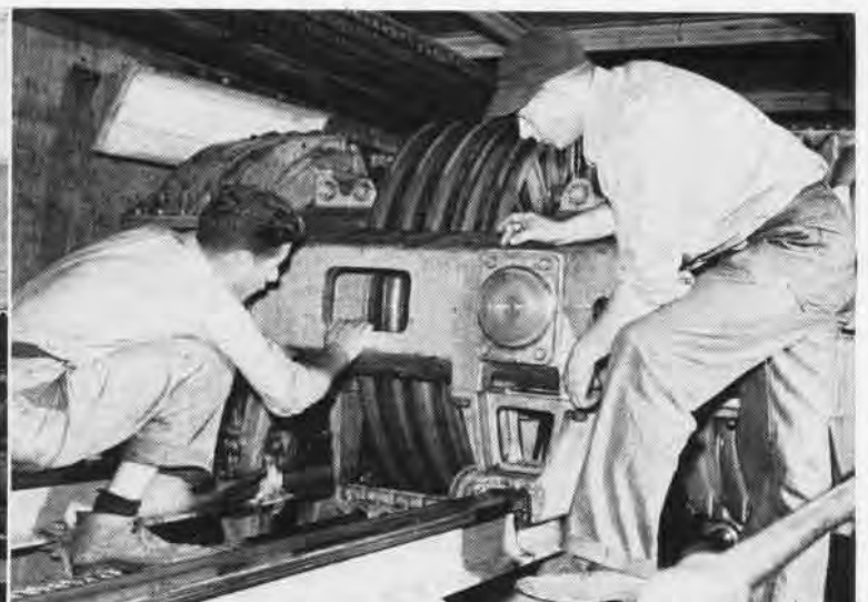
Students at catapult school at NAF, Philadelphia, disassemble piston valve on an H2 catapult. School is the only one to train such men
