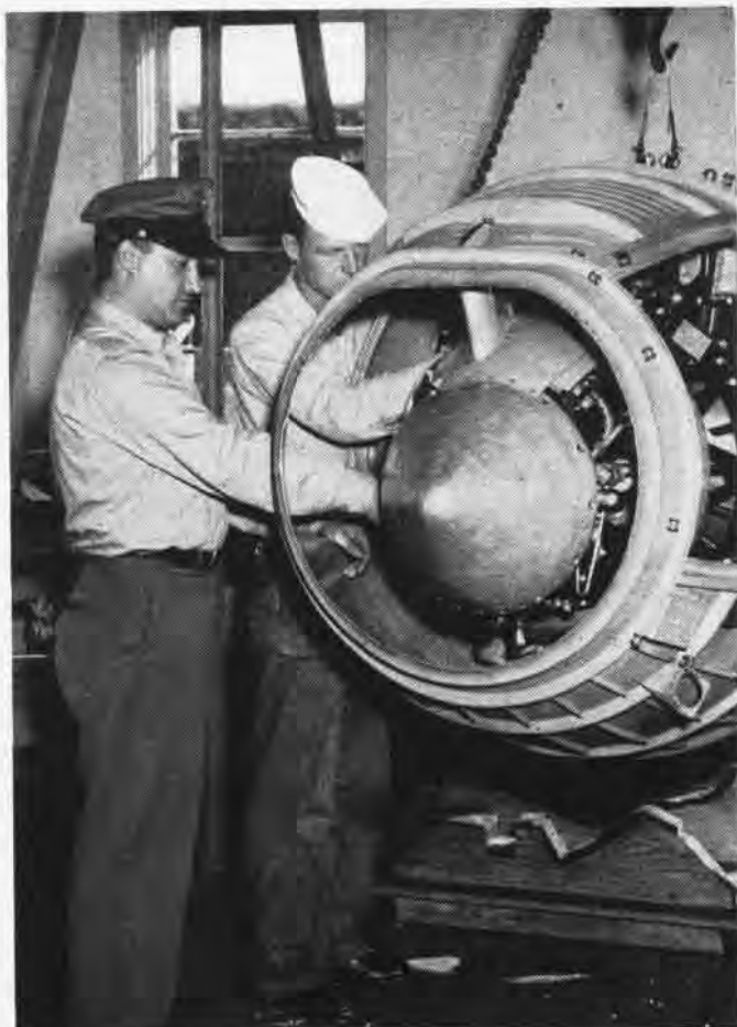
No Propeller in the way for these mechanics. Oil cooler installations become a thing of the past and involved maintenance is history
