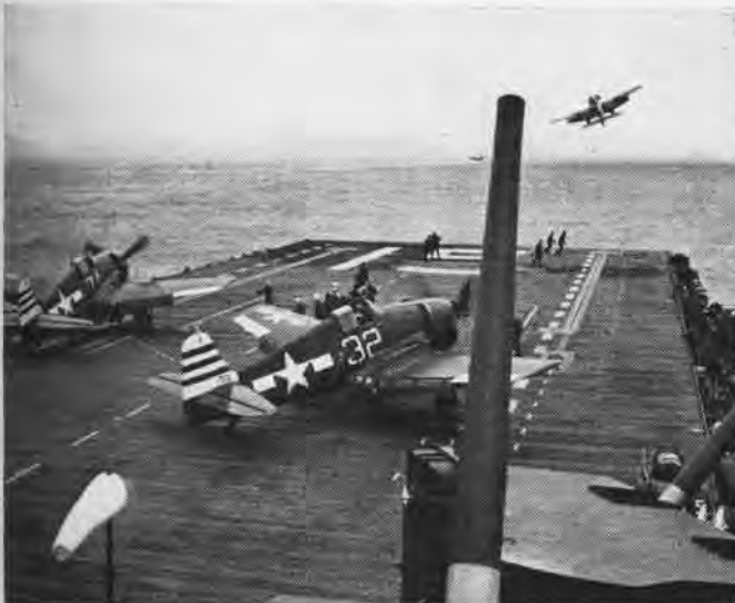
Randolph launching Hellcats for July raid on Jap homeland shows how a carrier catapults planes rapidly with only few seconds between
