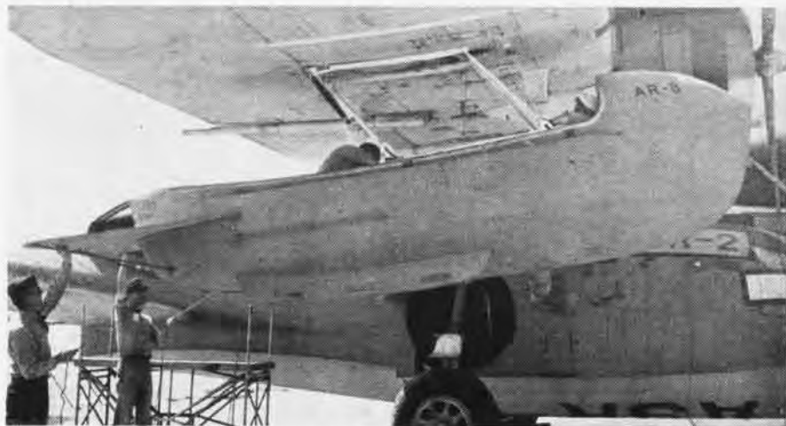
THREADED RODS AID IN SECURING AR-8 TO INBOARD BOMB RACK OF A NAVY CATALINA
