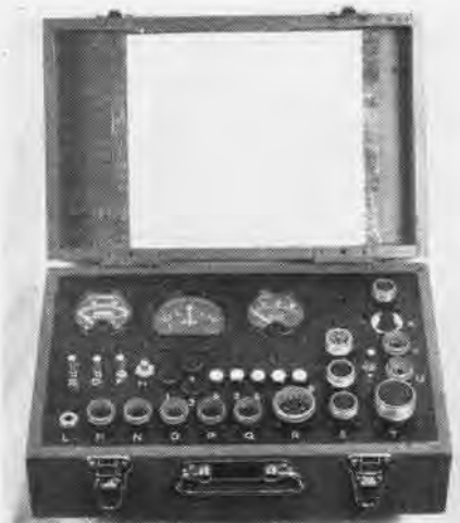
TEST UNIT OPERATES ON 26-VOLT CIRCUIT
