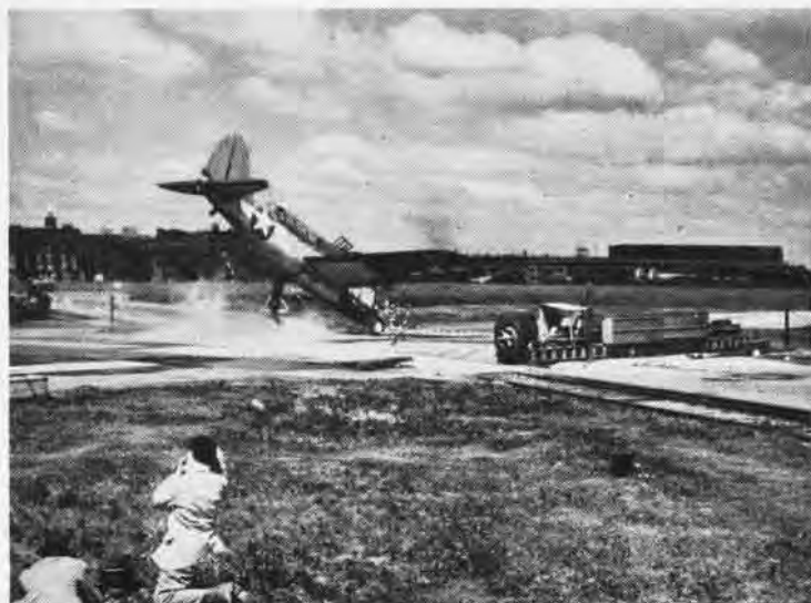
Surveyed SB2A tests barrier cable suspension at NAF, being catapulted against it. Mobile arresting unit (Morest) can be seen on right
