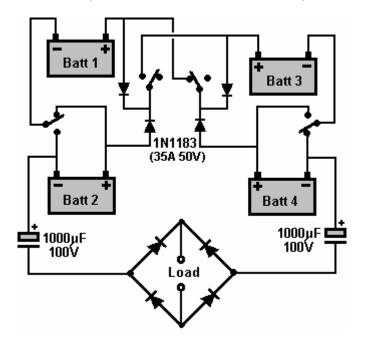
The simple circuit shown here was used by testers of the Electrodyne Corp. over a period of three years using ordinary vehicle lead-acid batteries. During that time, the batteries were not only kept charged by the circuit, but the battery voltage climbed to as much as 36 volts, without any damage to the batteries.
