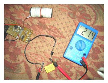
This is the first step in the process as the same circuit can be used to drive many coils of this type. The resistor feeding the base of the transistor is about 500 ohms for the prototype, but using a 390 ohm resistor in series with a variable resistor of say, 1K, would allow a good standard resistor value to be selected for each transistor/coil pair:
