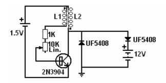
Coils: 0.5 to 1.0mm diameter solid copper wire length: 1 to 2 metres bi-filar wound
