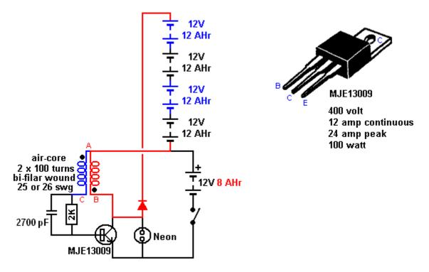
The coil is wound on a hollow former, using two separate strands of wire of 0.5 mm diameter, giving a resistance of just 2 ohms. The strands of wire are placed side by side in a single layer like this:
