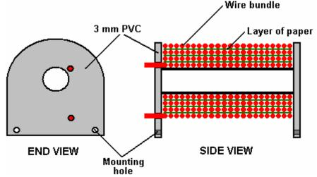
The coils are wound with the end plates attached and drilled ready to screw to their 1/4 inch (6 mm) PVC bases, which are the bolted to the 3/4 inch (18 mm) MDF supporting structure. To help the winding to remain completely even, a piece of paper is placed over each layer of the winding:
