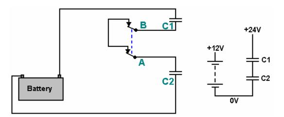
Here, the two charged capacitors are disconnected from the opposite supply rails and connected together to form a combined voltage of, in the case of a 12 volt battery, 24 volts connected across the 12 volt battery. This will cause a sudden inflow of current into the battery. However, before practically any capacitor current has flowed, the relay is operated again, repeating the sequence.
