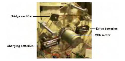
With this arrangement, one pair of AA-size NiCad batteries drives the motor, spinning the motor, moving its magnets rapidly past the ring of converted relays, producing charging DC current via the bridge rectifiers and that current is sufficient to keep the device running continuously.
