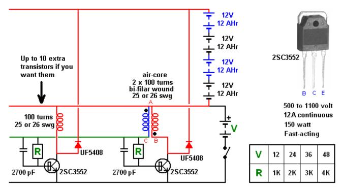
The 2700 pF capacitor is recommended for each additional transistor, but it is not an essential item and the circuit will operate ok with just the one on the bi-filar coil drive section.
