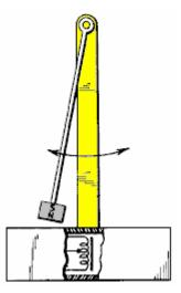
Andrews also shows a switching arrangement for a motor. This design is essentially the same as used by John Bedini in many of his pulsing systems:
