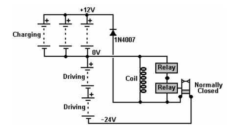
When using one of these relay charging systems you will find that quite a lot of noise is generated. This can be reduced quite easily with a little padding and it does have the advantage of indicating that the charging system is running correctly.
