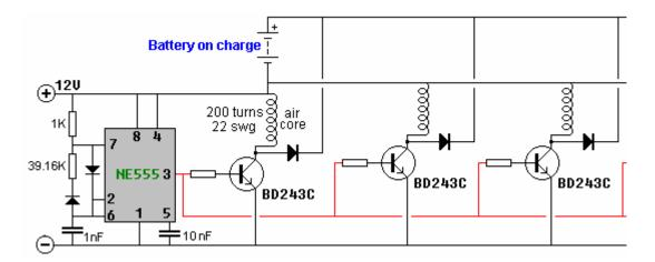
As can be seen from the photographs, Alex uses preset resistors to adjust the settings to their optimum values. The simplicity of this circuit makes it very attractive as a construction project and using more than one coil should make for impressive performance figures. Alex says that the best results are achieved with just the one (1000V 10A) diode and not a diode bridge, which is borne out by the teaching comments on the above web site.
