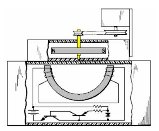
Here, as the rotor magnet passes the curved electromagnet in the base, it switches on the two transistors which produce a pulse which keeps the rotor spinning and the tiny generator turning. Andrews produced this for amusement as the rotor appears to spin on it's own without any drive power.
