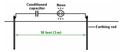
I use a very low-powered high-voltage source with a power output of only 1.2 watts as I like to play safe with these things. With a low power source, I have charged batteries using pulses of up to 800 volts without the batteries showing any ill effects. Also, using one-wire electricity is safer as that transmits mostly voltage and so minimum current is fed. So, to condition a battery or a capacitor using cold electricity, you can use a circuit like this:
