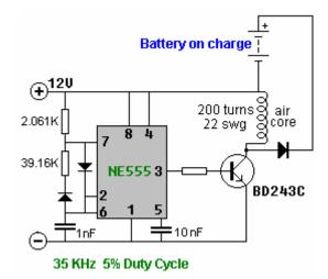
Here, the coil is wound with 200 turns of 0.7 mm enamelled copper wire and the actual construction is compact:
