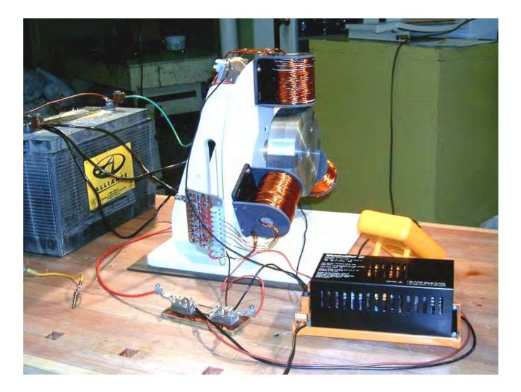
This is not a toy. It draws significant current and produces substantial charging rates. This is how Ron chose to build his device. The rotor is constructed from aluminium discs which were to hand but he would have chosen aluminium for the rotor if starting from scratch as his experience indicates that it is a very suitable material for the rotor. The rotor has six magnets inserted in it. These are evenly spaced 60 degrees apart with the North poles all facing outwards.
