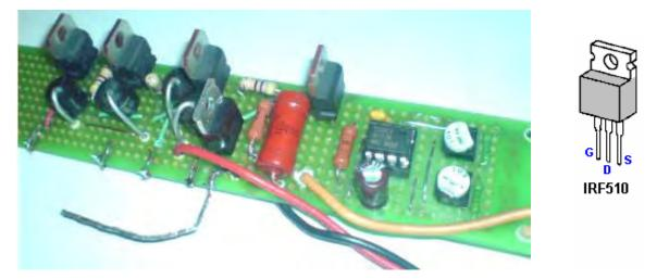
It is possible to use various different transistors with these circuits. As some people have difficulty in working out a suitable physical construction for a circuit, here is a suggestion for a possible layout using an MJ11016 high-power high-gain transistor on stripboard.
