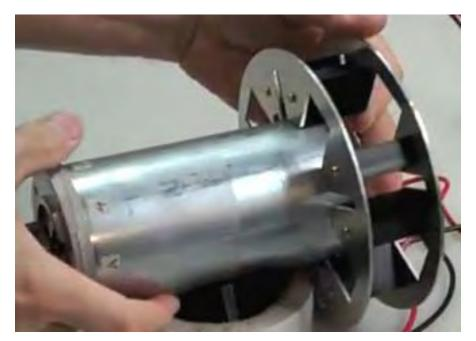
The frame is made from two pieces of 3 mm aluminium with plastic spacers holding the two aluminium discs apart. The plastic spacers are secured with brass screws. As the motor casing is about 3 mm thick steel, that tends to deflect the added magnetic field outwards, which is the reverse of what is wanted. So, a 6 mm thick strip of steel is placed outside the magnets in order to direct the field inwards. The magnets and steel strips are then inserted to complete the arrangement:
