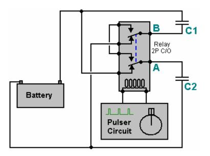
Here, the pulser circuit is set to give short, very sharp pulses to drive the relay cleanly. The relay has two changeover contacts "**A**" and "**B**". The operation is very simple. Initially, the capacitors "**C1**" and "**C2**" are charged up when the relay is in it's unpowered state and no current is flowing through the relay coil:
