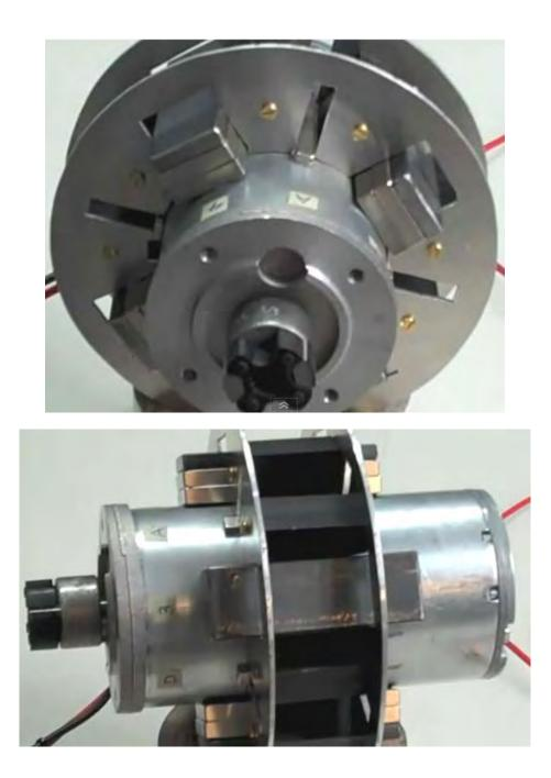
The motor is demonstrated when set up like that. Then four sets of very narrow magnets are added in intermediate positions and the number of broad magnets increased to three at each location, the steel strips discarded and four broad magnets used at each of the four locations around the motor:
