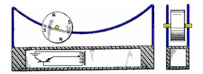
It operates in almost the same way, with a magnetic wheel rolling backwards and forwards along a curved track. At the lowest point, the electromagnet is triggered by the induced voltage in some of the turns of the coil, powering the transistor and boosting the magnetic roller on it's way.
