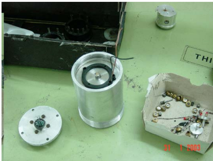
Figure IV.IX.XIV - Al Fatah impact fuse dismantled at the Nissan facility
