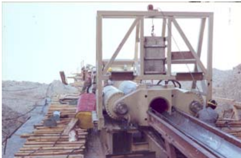
Figure IV.VII.IV Rear part of the fixed, 45°inclined Supergun System
