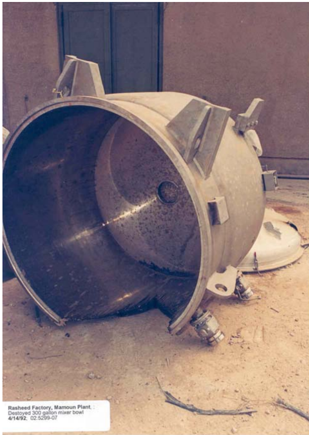
Figure IV.II.XXXI 1200 litre propellant mixer bowl destroyed under UN supervision
