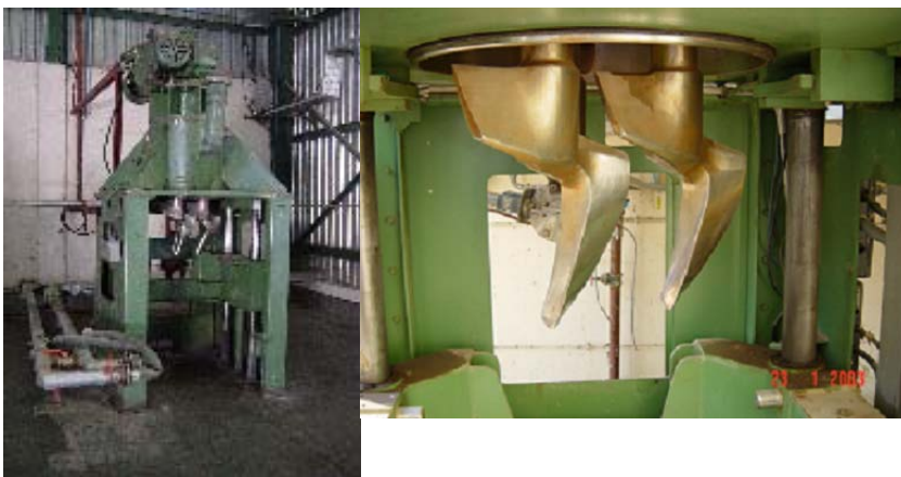
Figure IV.IX.XXXVIII - A 120 litre three-blade mixer used for Al Fatah motor production – Al Mamoun
