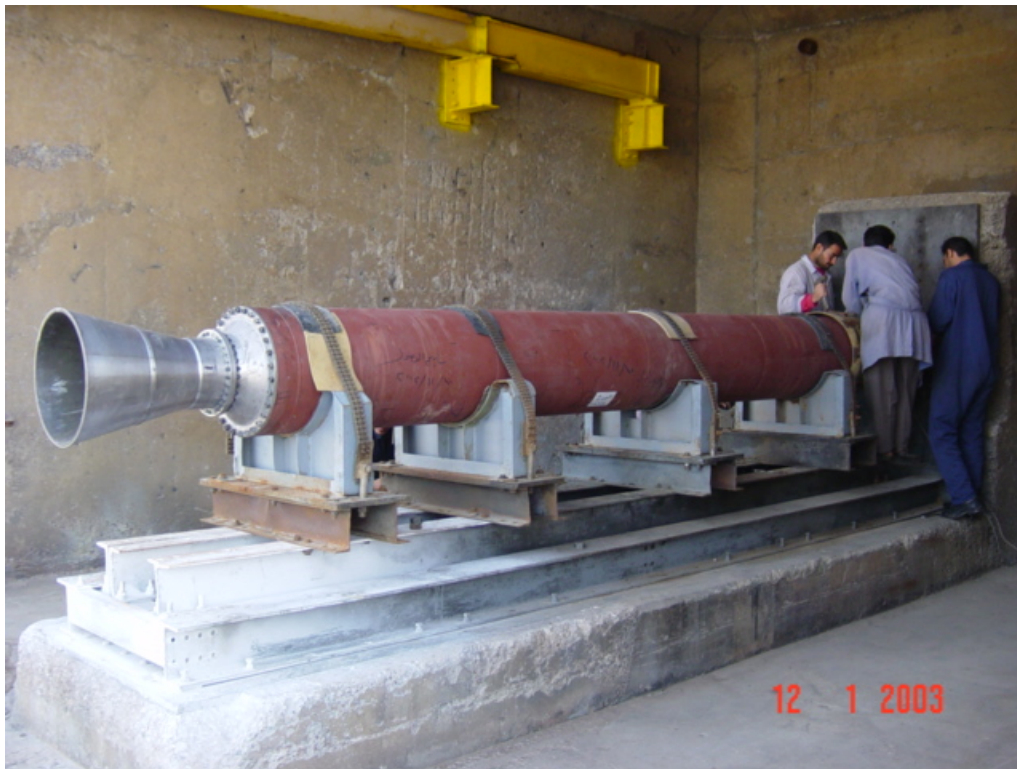
Figure IV.IX.LV - Al Ubour Static Test at Al Mutassim
