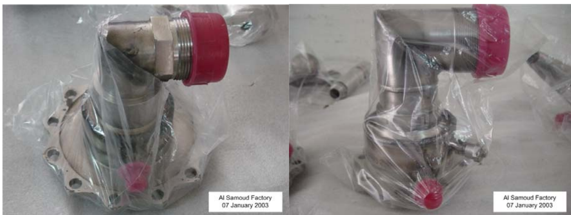
Figure IV.VIII.LV - Turbo pump Fuel (left) and Oxidiser (right) Intakes (Al Samoud Factory)
