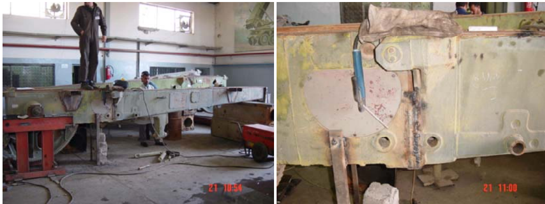
Figure IV.IX.XLVII - SA-2 modified launcher (left - with support for canister; right - detail of welded breaking mechanism) - Al Feeda, 21 11 2002
