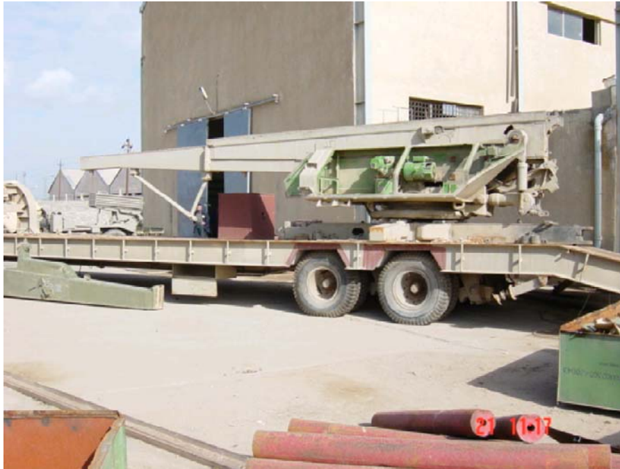
Figure IV.IX.XLVIII – SA-2 modified launcher on the tank transport trailer.
