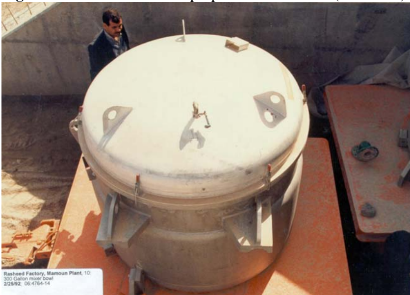
Figure IV.II.XXX 1200 litre propellant mixer bowl (one of six).
