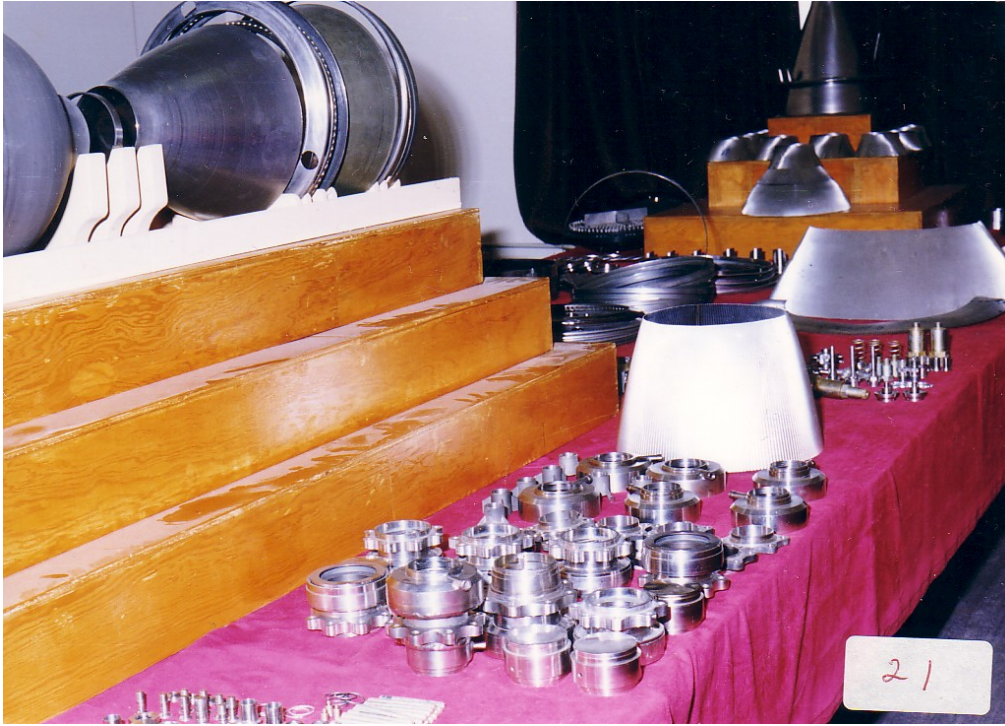
Figure IV.III.XLIV. Turbo pump parts for a SCUD-B engine produced by Project 1728.
