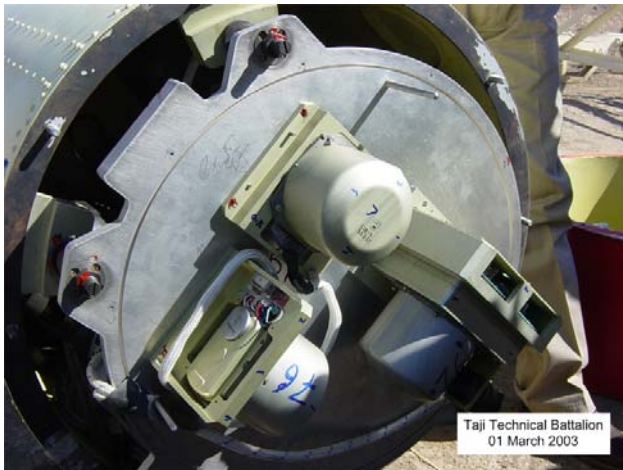
Figure IV.VIII.XXVIII - Front of fuel tank section equipped with gyroscope platform (Taji Technical Battalion)
