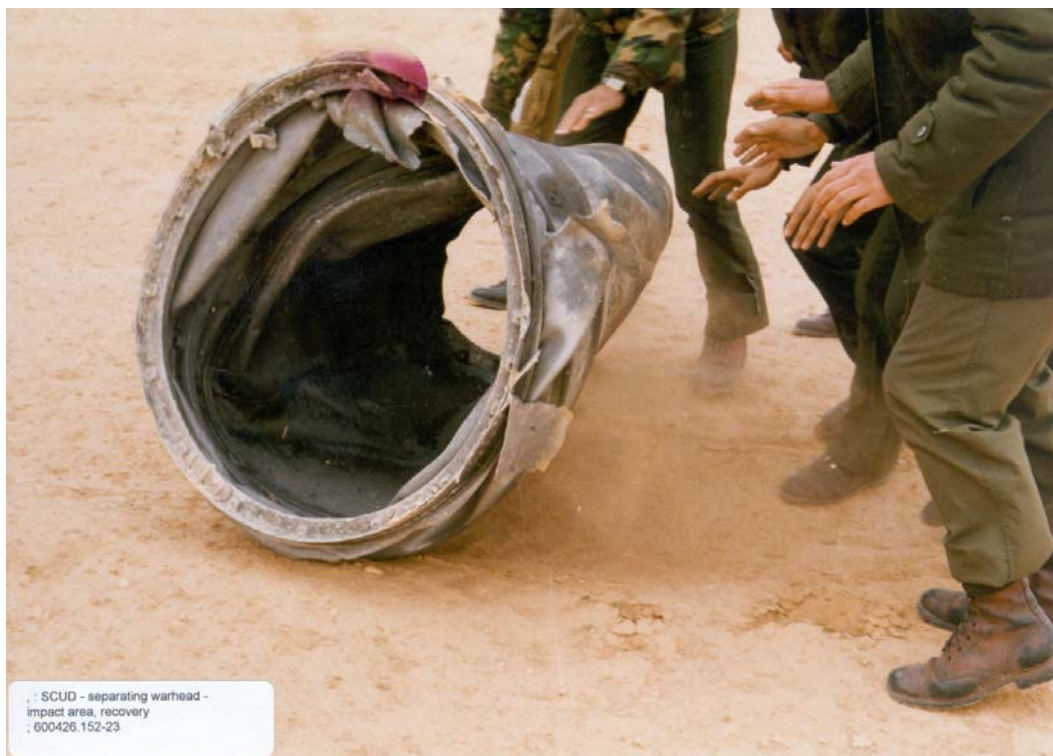
Figure IV.III.XVII Separable warhead equipped with linear charge recovered after flight test - rear view. (Haidar farm photo)
