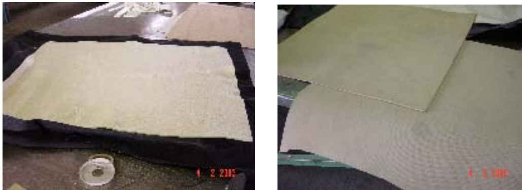
Figure IV.IX.XXXII - Insulation sheet before and after hot pressing – Al Mamoun
