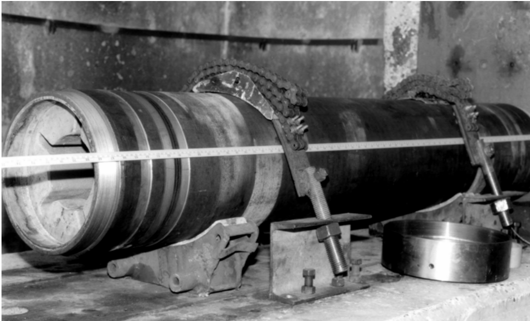
Figure IV.IX.III – Sub-scale Ababil-100 motor on static test bench
