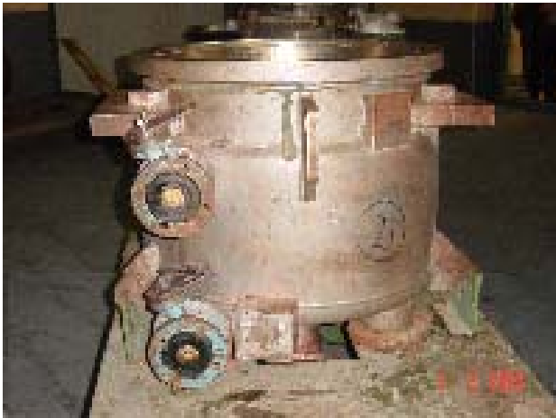
Figure IV.IX.XXXVIII - A 120 litre three-blade mixer used for Al Fatah motor production – Al Mamoun
