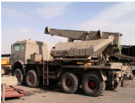
Figure IV.IX.XLIX- SA 2 modified launcher (support for canister) on the bed of a truck - Al Feeda, 21 Nov 2002
