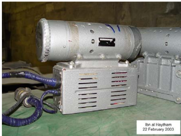
Figure IV.XI.XX - SA-2 electromechanical inverter
