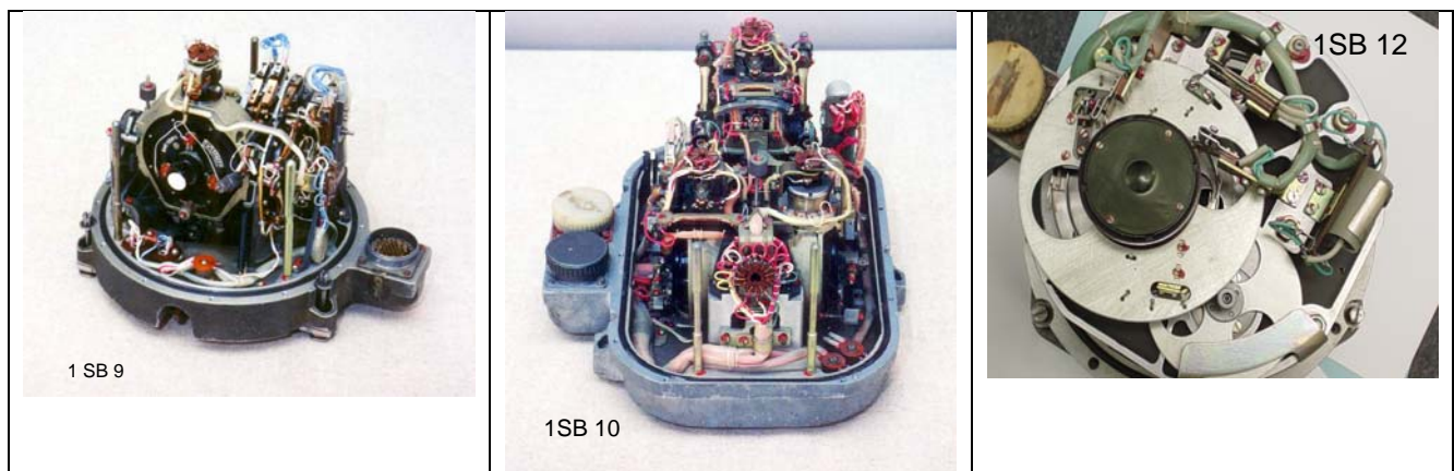
Figure IV.XI.II - SCUD gyro sensors subsystems
