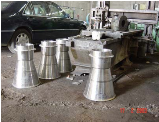
Figure IV.IX.XXIX - Divergent sections after machining
