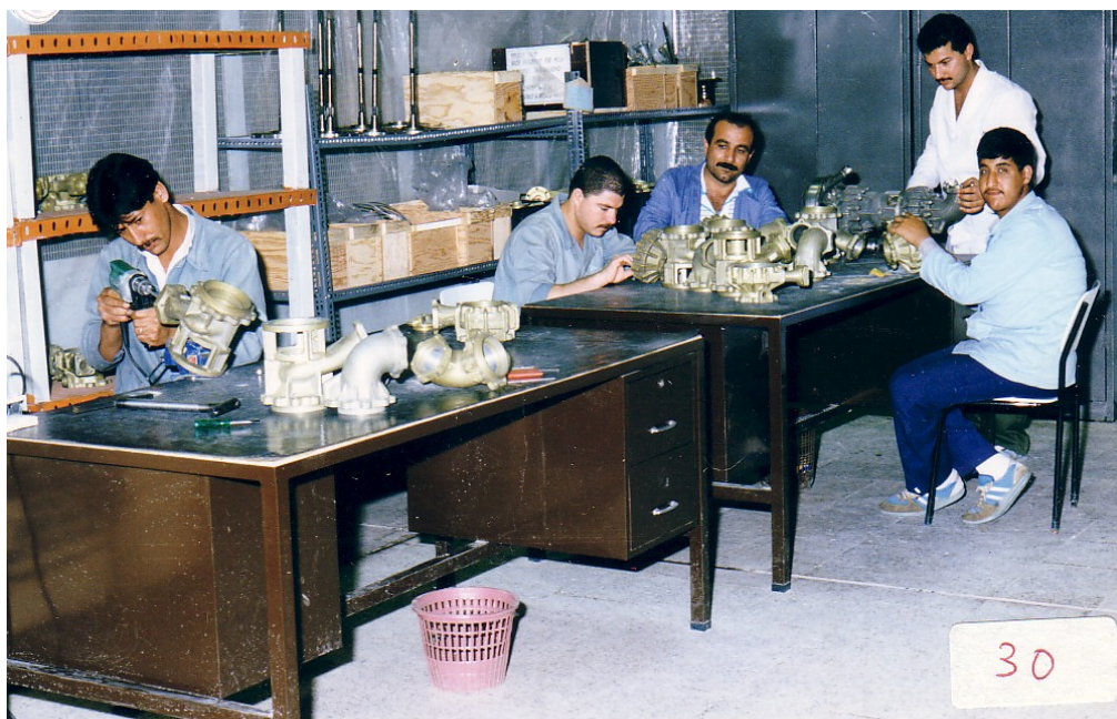
Figure IV.III.XLV. Workers assembling turbo pumps in Project 1728.
