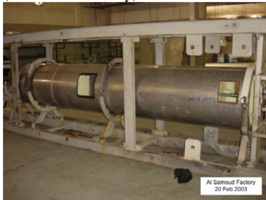
Figure IV.VIII.XXXVIII - Alignment of fuel and oxidiser tank sections (Al Samoud Factory)
