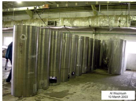
Figure IV.VIII.XXXIV - Oxidiser tanks under manufacture (Al Waziriyah)
