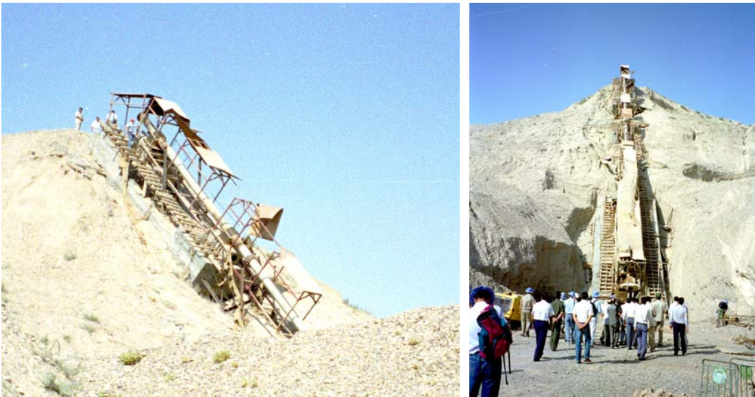
Figure IV.VII.III The Fixed, Inclined Supergun System (350 mm diameter and 52.5 metres long)
