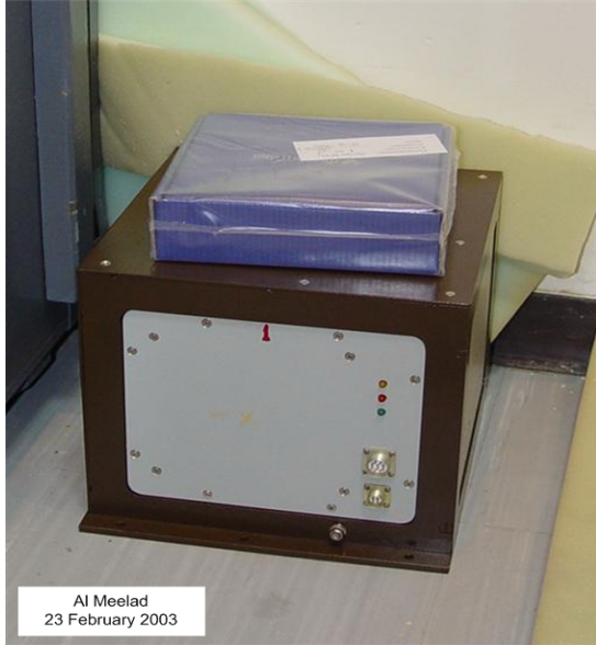
Figure IV.XI.LIII A-16 accelerometer and power supply unit of FOG INS (Al Meelad February 2003)
