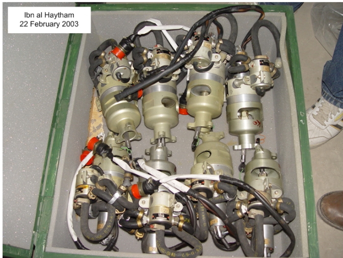
Figure IV.XI.XXII - SA-2 (20 DSU) actuators used on operational Al Samoud-2 missiles
