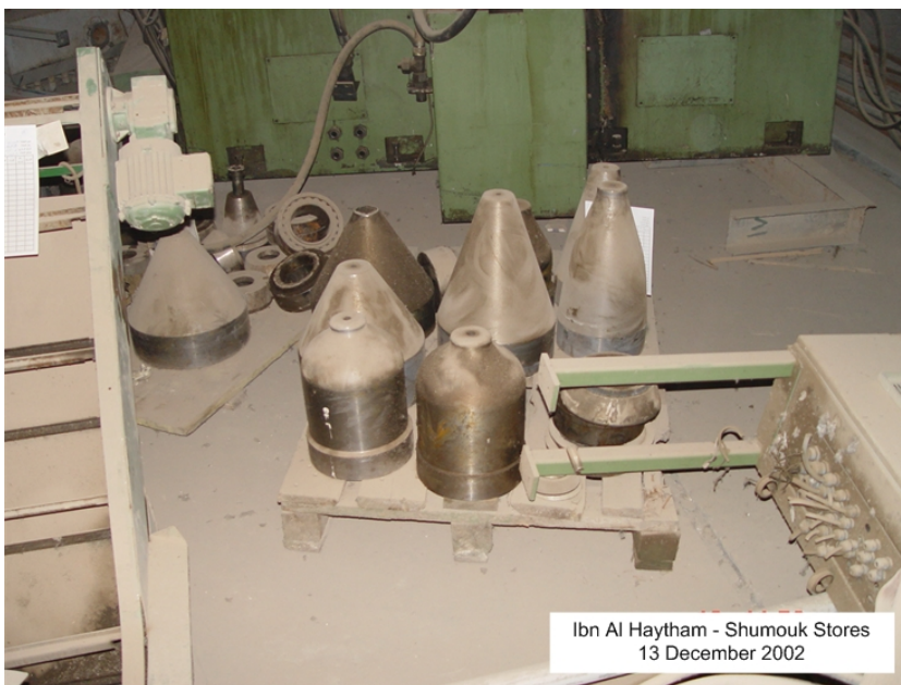
Figure IV.VIII.LI - Flow forming dies/moulds for liquid propellant engine production (Shumouk Stores)
