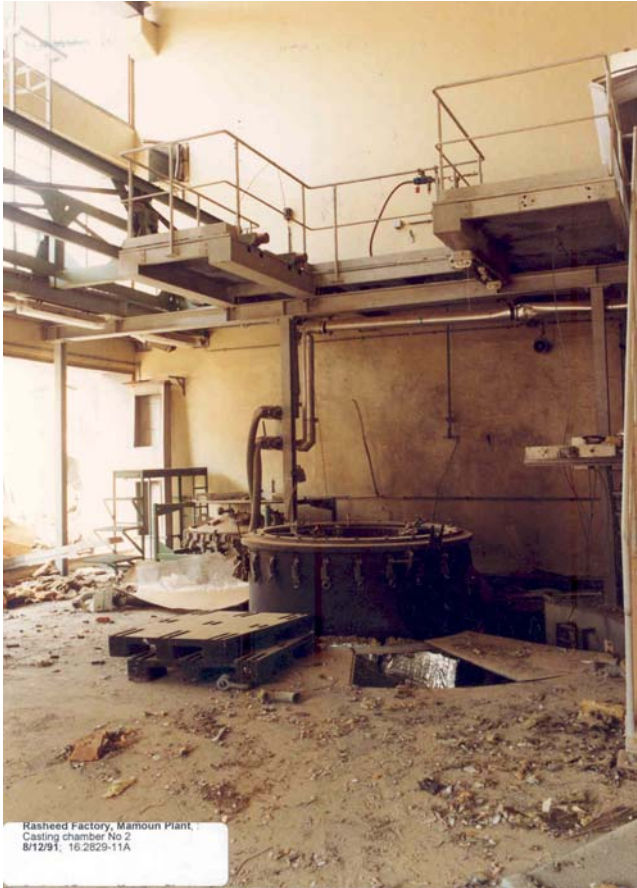
Figure IV.II.XXXIV. (a) BADR-2000 casting/curing chamber no. 2 in building 162 (17).
