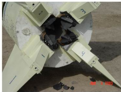
Al Samoud 2 Jet Vanes destroyed by hammer
