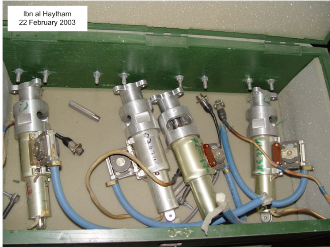
Figure IV.XI.XXII - SA-2 (20 DSU) actuators used on operational Al Samoud-2 missiles
