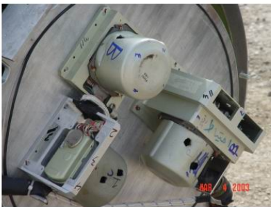
Al Samoud 2 Gyroscopes destroyed by pickaxe
