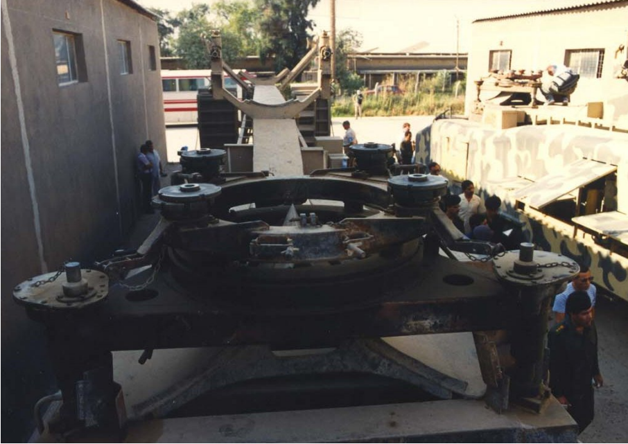
Figure IV.III.XXXVI Fixed launcher type arm mounted on flatbed trailer for Al Nida mobile launcher
