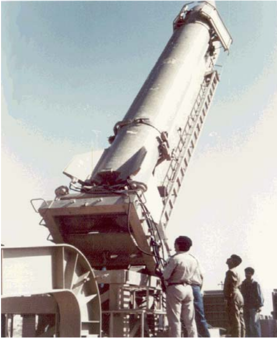
Figure IV.III.XXXVIII Al Hussein missile being erected on Al Nida launcher.
