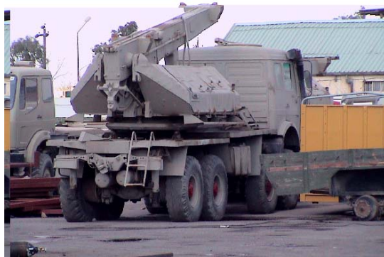
Figure IV.IX.XLIX- SA 2 modified launcher (support for canister) on the bed of a truck - Al Feeda, 21 Nov 2002
