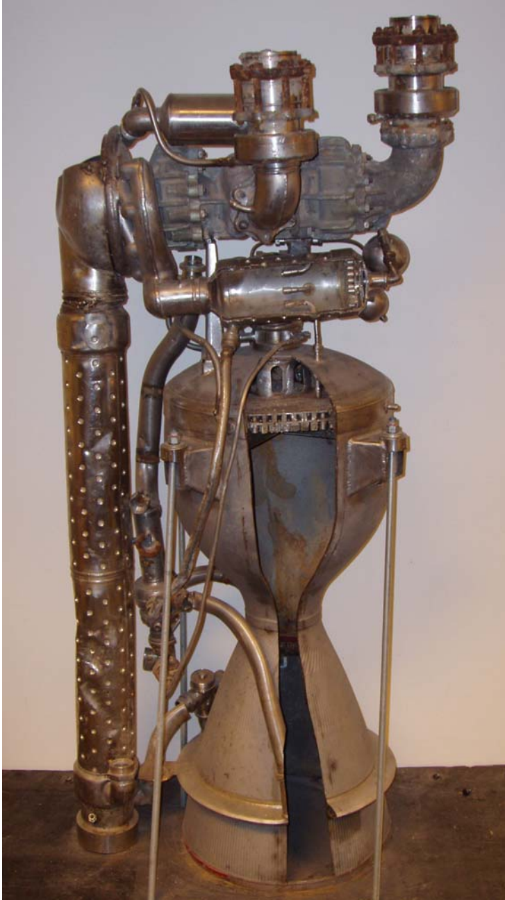
Figure IV.III.XXIX. A SCUD-B liquid propellant engine (showing cut-away section of combustion chamber and nozzle)
