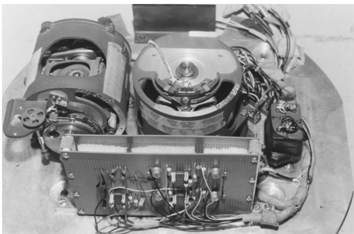
Figure IV.XI.IV - Assembly of modified HY-2 yaw and roll gyroscopes
