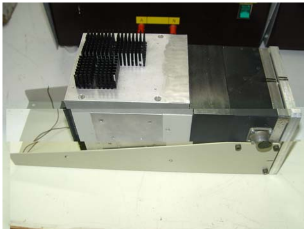
Figure IV.XI.XXXVI - Imported INS composed of 2 MG-4 Gyros (two channel each), 3 A-15 Accelerometers and related electronics circuit.
