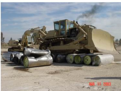
Propellant tank destruction
