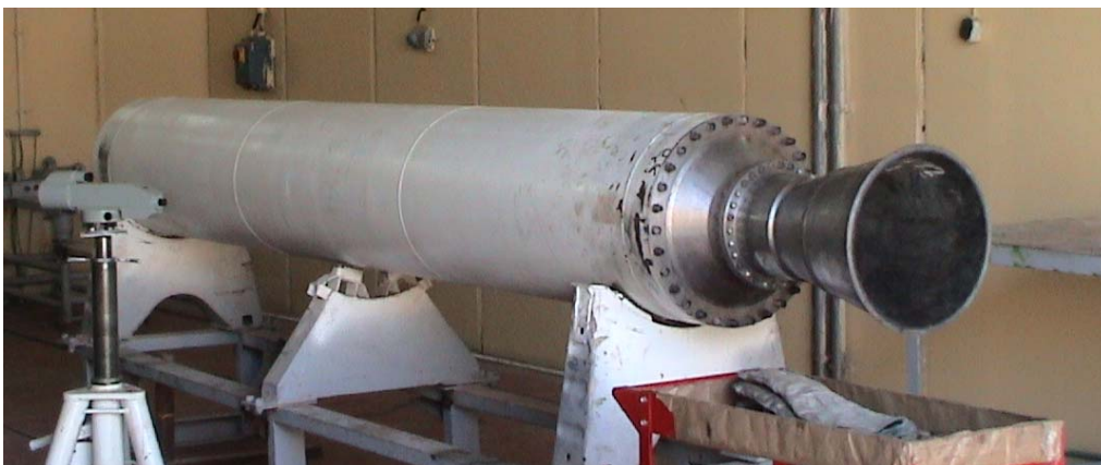
Figure IV.IX.XIX - Al - Fatah motor in final assembly stage
