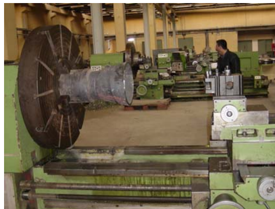
Figure IV.IX.XXVIII. Machining divergent sections
