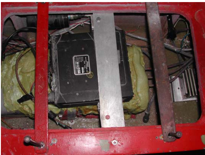
Figure IV.X.IX Fuel tank in RPV-20 (under data recorder and layer of foam)
