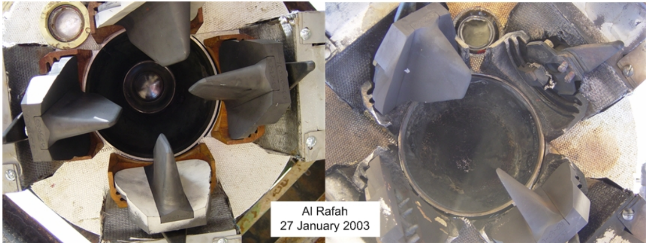
Figure IV.XI.XXIII - Al Samoud-2 graphite jet vane test (before and after test)
