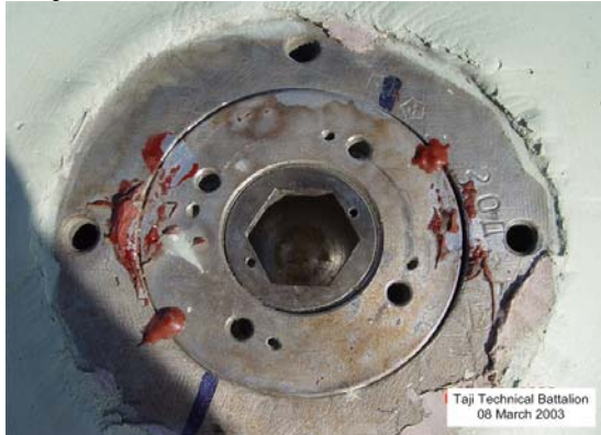
Figure IV.VIII.XXXV - Oxidiser tank filler cap (scavenged from SA-2 missile) (Taji Technical Battalion)
