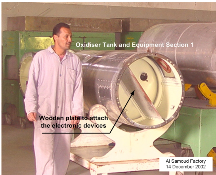
Figure IV.VIII.XXXII - Oxidizer Tank and Equipment Section 1 (Al Samoud Factory)
