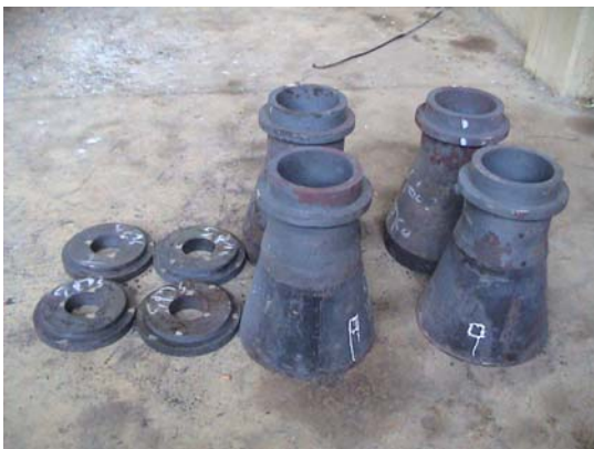
Figure IV.IX.XXVII. Forged and welded divergent sections.
