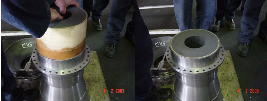
Figure IV.IX.XXXV - Insertion of carbon throat in the nozzle
