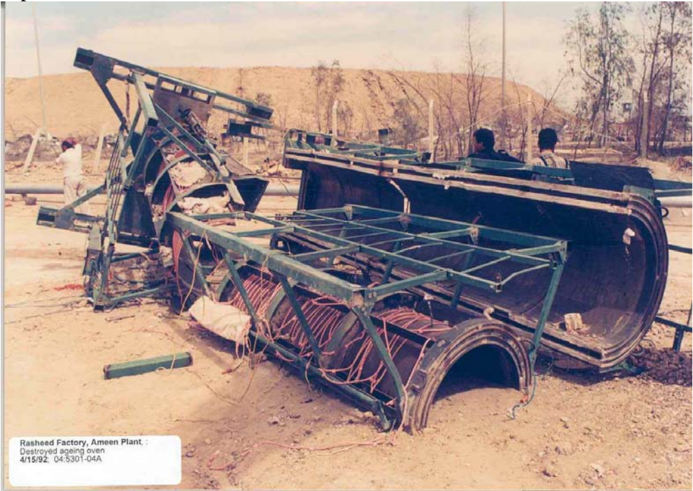
Figure IV.II.XLIX Annealing oven for BADR-2000 motor case destroyed under UN supervision.
