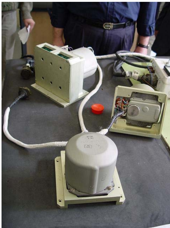
Figure IV.XI.XIV - SA-2 two-degree of freedom gyroscopes used for Al Samoud-2
