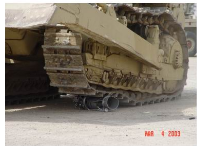
Al Samoud 2 Engine crushing
