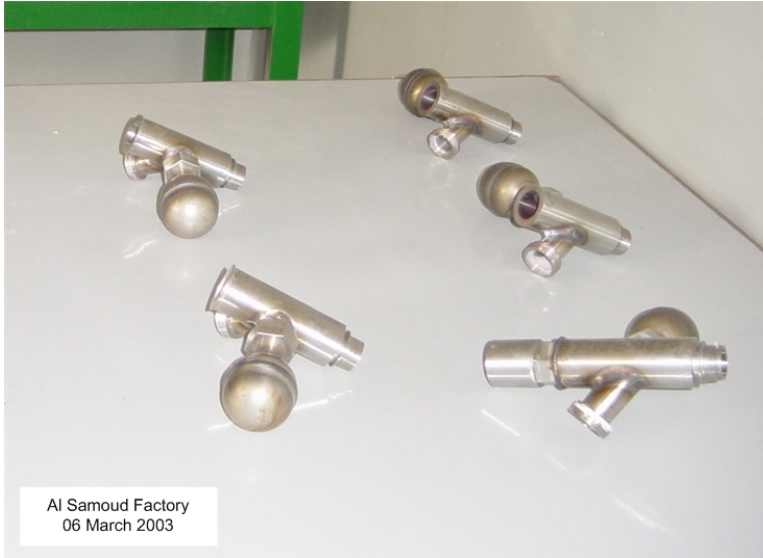
Figure IV.VIII.LVIII- Al Samoud shut-off valves (Al Samoud Factory)
