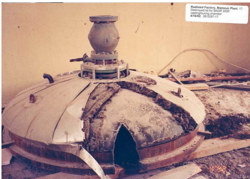
Figure IV.II.XXXV BADR-2000 casting/curing chamber lid; destroyed under UN supervision.
