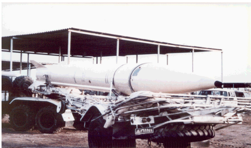
Figure IV.III.XXXII Unmodified SCUD-B on unmodified trailer
