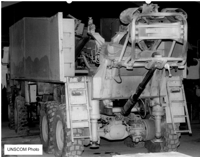
Figure IV.VIII.LXI - Al Samoud-2 launcher version 1 (Al Fedaa Factory)
