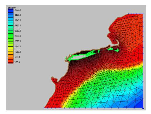
Figure 6. Domain of the ADCIRC model showing the varying size of the triangular grids according to the detail needed to simulate the hydrodynamics.
