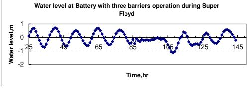
Figure 9. Closing the three barriers during Super Floyd lowers the water level inside the barriers to approximately mean sea level.
