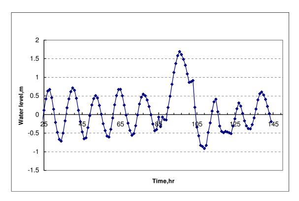
Figure 13. With two barriers closed and the East River open during Super Floyd, the peak water level is higher than if all three barriers were open.
