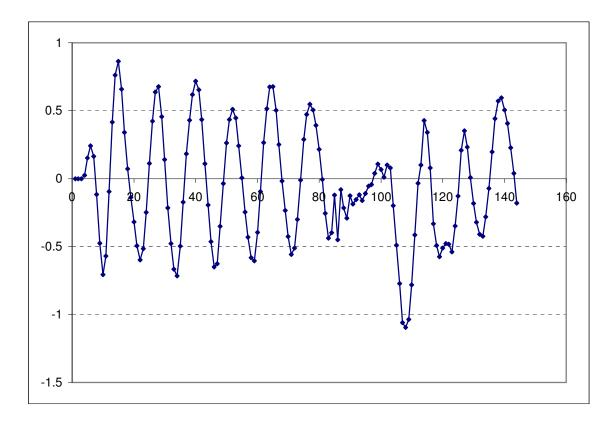
Figure 17. The SBSS simulation indicates that the water level behind the barriers would have risen about 0.25 meters due to the inflow from rain-swollen rivers during the 20 hours the barriers were closed in Tropical Storm Floyd.
