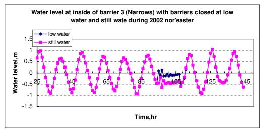
Figure 10. In the 2002 nor'easter, closing the barriers at slack water leads to lower water levels behind the barriers than if they were closed at low water.
