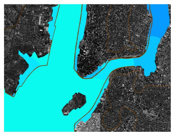
Figure 14. Superposition of Super Floyd flooding predictions and aerial photographs of lower Manhattan and environs.
