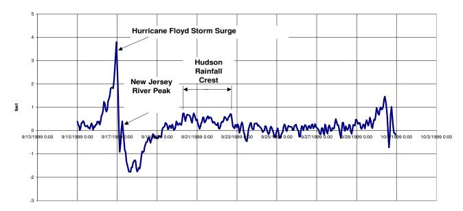
Figure 16. Deviations from normal tide levels at the Battery due to Tropical Storm Floyd.
