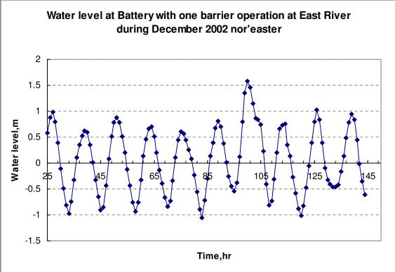
Figure 11. With a single barrier, located in the East River, the storm surge from Long Island Sound is stopped, but the water elevation west of the barrier nevertheless reaches flood level.
