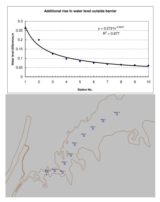
Figure 12. Pushed against the closed East River barrier in the 2002 nor'easter, the water level rises an additional 0.27 meters. However, this additional rise diminishes exponentially with distance from the barrier, dropping by about one-third at Willets Point.
