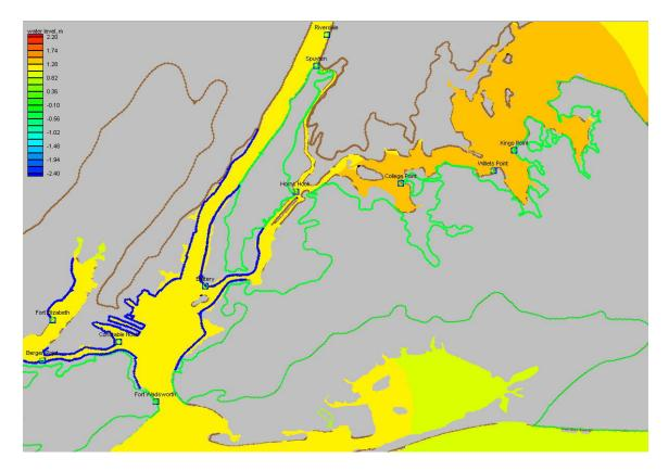
Figure 15. Without barriers in place, Super Floyd would cause coastal flooding in many areas within the central metropolitan region.
