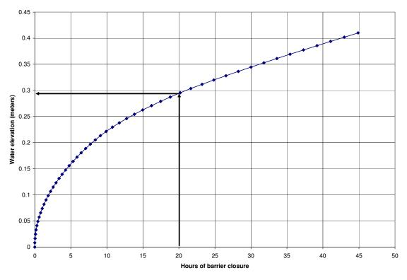
Figure 18. Considering only the storage volume above the upward sloping Hudson River, the rainfall runoff crest would raise the water level behind the barriers less than 0.3 meters during the 20 hours that they would have been closed for Tropical Storm Floyd, and less than 0.4 meters in 40 hours.
