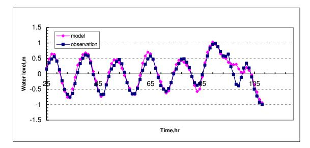
Figure 8. The SBSS simulated values of water level at the Battery closely match those actually observed in Tropical Storm Floyd through the storm surge peak.
