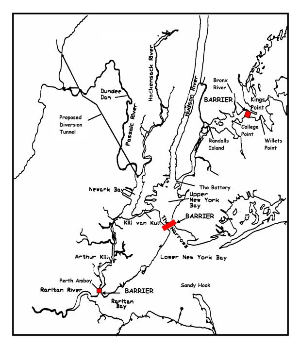
Figure 3. The waterways surrounding New York City can be protected from coastal flooding with three barriers. Figure adapted from Cerco, C.F., B. Bunch, and J. Letter. Impact of flood-diversion tunnel on Newark Bay and adjacent water, Journal of Hydraulic Engineering, April 1999.
