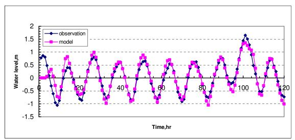
Figure 7. Ths SBSS simulated values of water level at the Battery during the December 2002 nor'easter closely match those actually observed.
