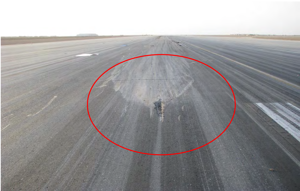
Figure 10: Tail Impact following Rupture of Fuselage
