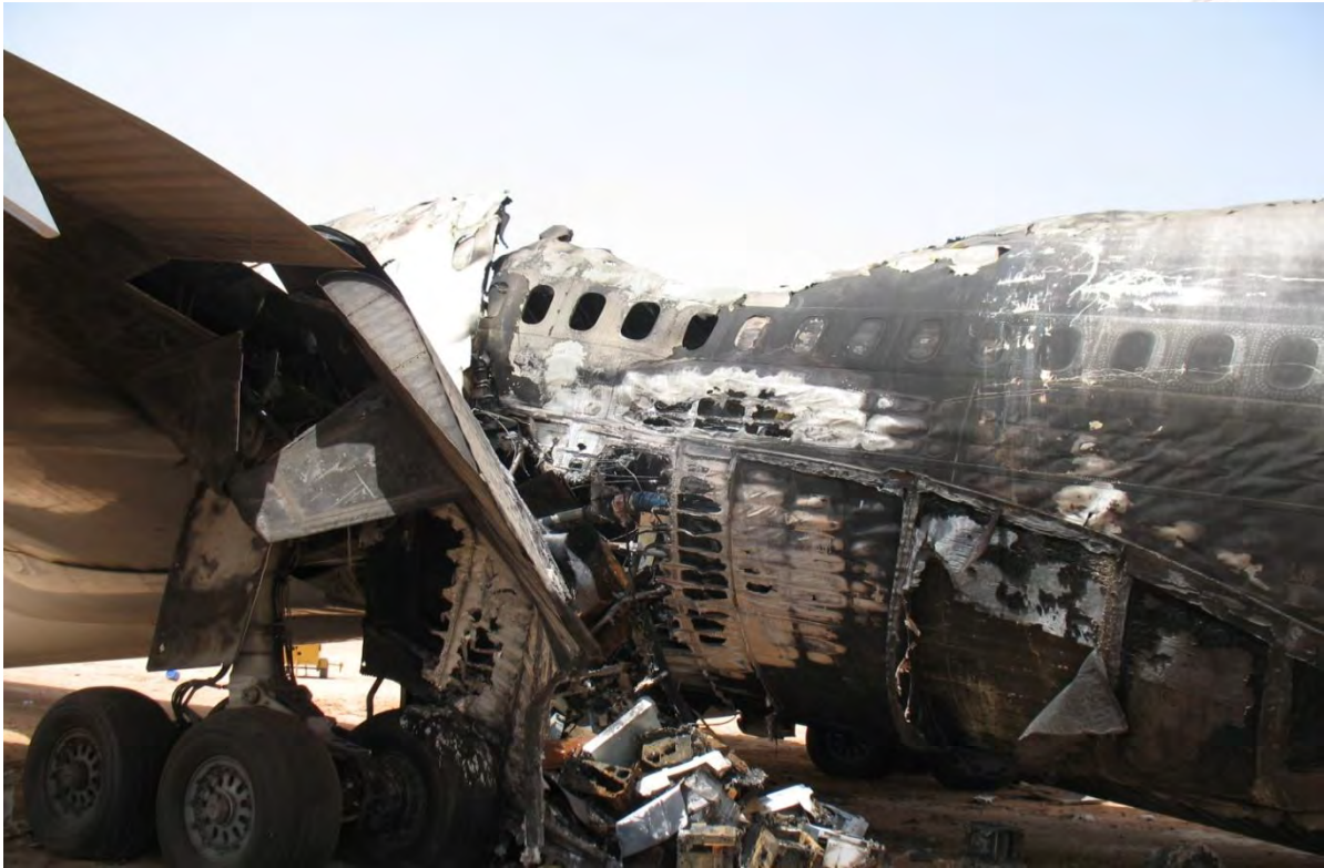
Figure 23: Area of Heaviest Fire Damage (Left Side)
