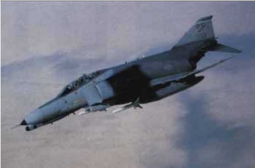
F-4G Wild Weasels, like this one from Spangdahlem AB, Germany, zeroed in on SAM guidance radars, and other aircraft hit early warning systems. Iraqis quickly learned to turn off radars, which virtually blinded the enemy force.
