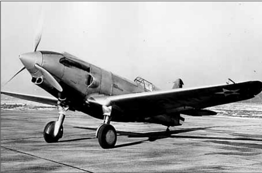
An unusually skillful pilot, Alison said if you could fly one airplane, you could fly them all. Among the lesser known aircraft he flew: a P-37 like this one, a variant of the radial engine P-36, designed around an Allison V-1710-11 engine.
