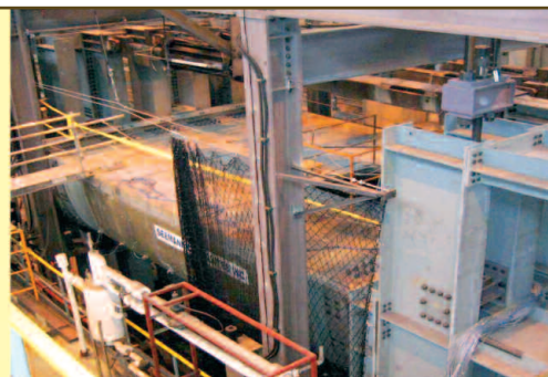
Above: Hull-girder bending tests conducted to determine the hull elastic behavior and its buckling and collapse strength.
