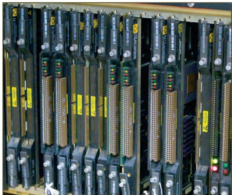
Right: The Input/Output Unit with system and user modules in place. Photo by Larry Hawkes, NSWC Carderock Division.
