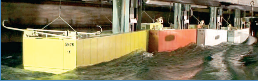
Seatrain units under tow at NSWCCD's David Taylor Model Basin. Combined hydrodynamic efficiency increases when units operate closely in tandem formation. Photo by Jesse Geisbert, NSWC Carderock Division.
