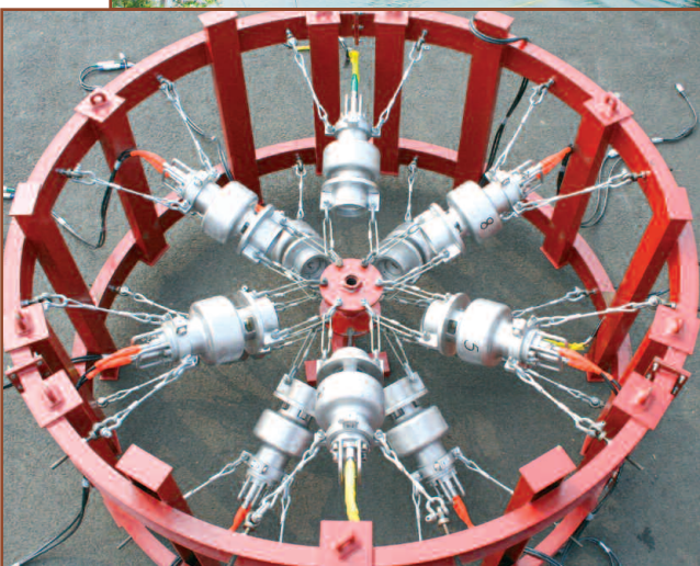
Left: A circular array of air guns. Unlike explosives, air gun arrays are placed close to a ship to impart shock energy.
