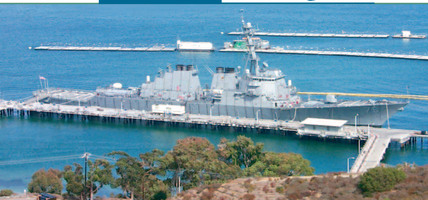
Above: USS Higgins in San Diego deperming slip. Note the perming coils wrapped around the exterior of the ship.
