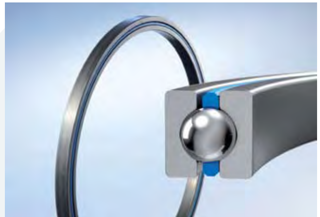
LEG 8: Slim bearing with 2 wire races and 4-point-contact.
