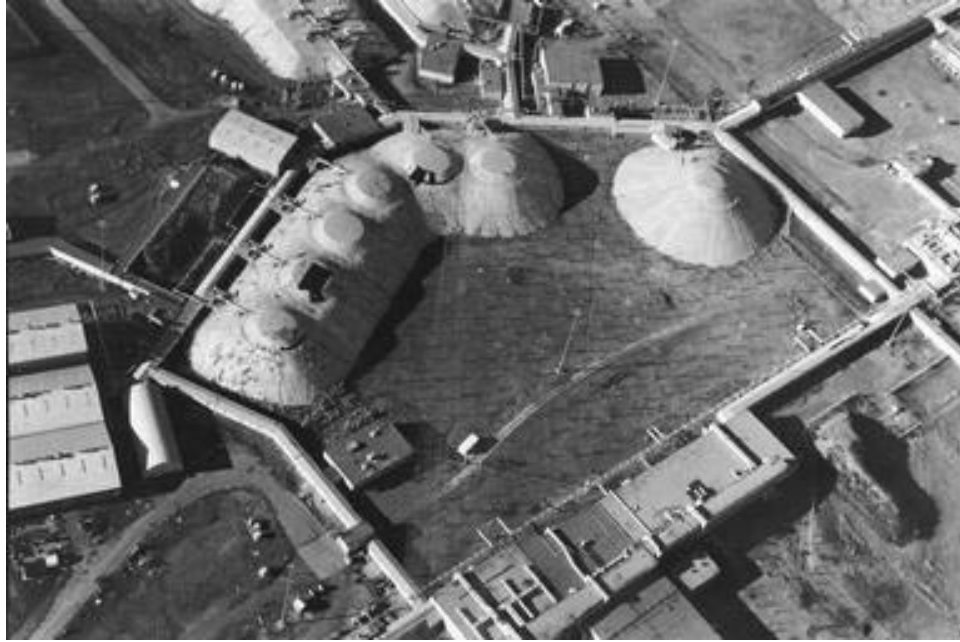
Fig. 25: Gravel gerties used for the assembly and disassembly of weapons cores.
