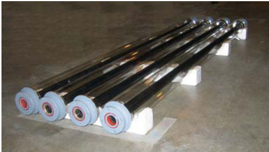
Figure 31. Heat Collection Element (HCE) receiver detail. Central receiver tube is coated with a dark paint, and surrounded by a vacuum-tight transparent insulating tube that is filled with a getter.
