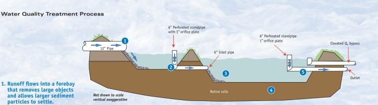
2. Runoff exits the forebay though a perforated standpipe and flows into the pond. When forebay capacity is reached, the overflow spills across a weir into the retention pond basin.
