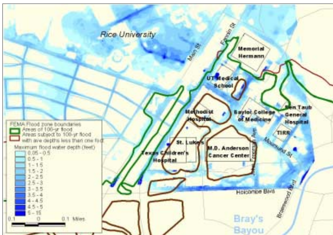
Figure 4. Flooding in the TMC was almost entirely caused by inadequate storm water drainage and resulting surface water build-up on streets. As shown in this image, flood depths of more than 5 feet (1.6 meters) were recorded on TMC streets.
