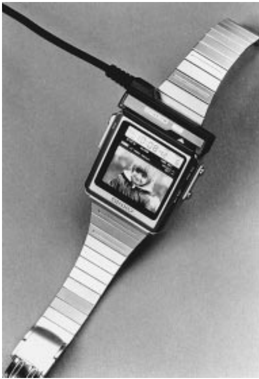
Fig. 52. Crystalline-Si-TFT blue-monochrome guest-host television watch worn by 007—Her Majesty’s Secret Agent. Courtesy of Seiko.
