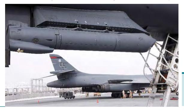
In foreground, a Sniper advanced targeting pod hangs from the underside of a B-1B bomber. Another B-1B is shown in the background. With the Sniper pod, the B-1B carrapidly switch into its so-called "ISR mode" and monitor the battle space. (USAF photo/SSgt. Darnell Cannady)
