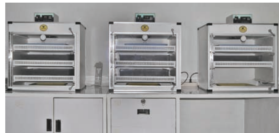
The incubators allow for three temperature regimes to determine if a TSD pattern exist for the Siamese Narrow-headed Softshell Turtle.
