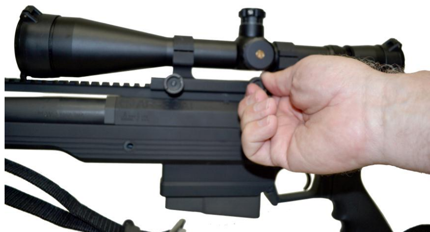
Attaching the ArmaLite® Scope Mount
