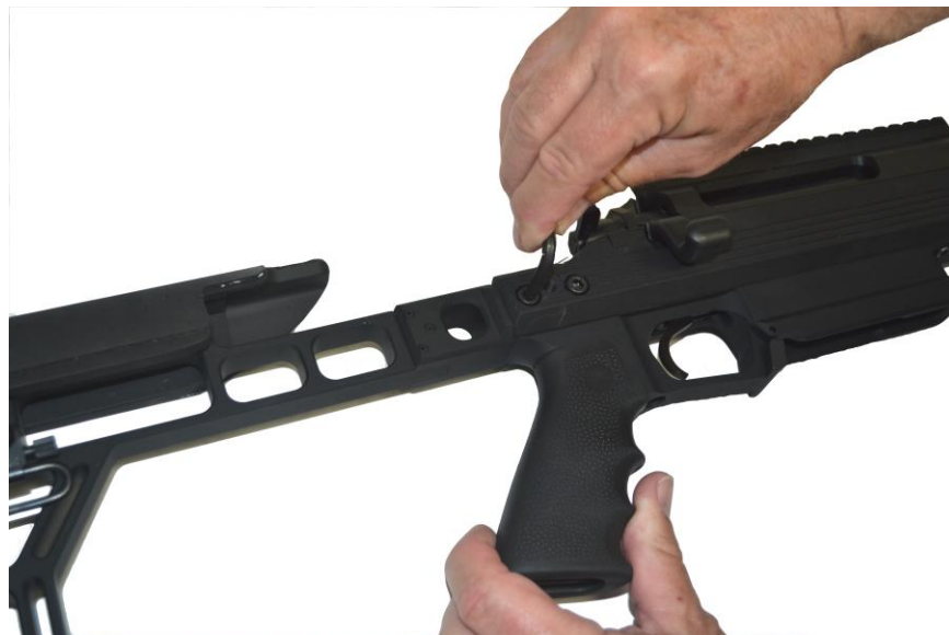
Removing the Buttstock
