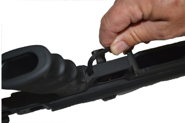
Removing the Grip Frame
