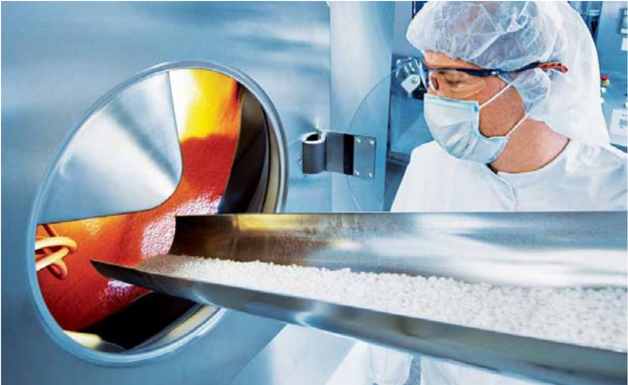
Bayer employee Frank Schaeff at the Xarelto™ tablet coating machine in the Leverkusen solids plant
