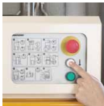
The baler has a simple control panel and is equipped with easily understood pictograms.
