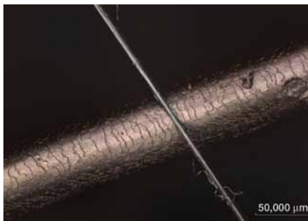
▲ Figure 6. Spider silk has a diameter of a few microns — roughly one-thirtieth the thickness of a human hair.
