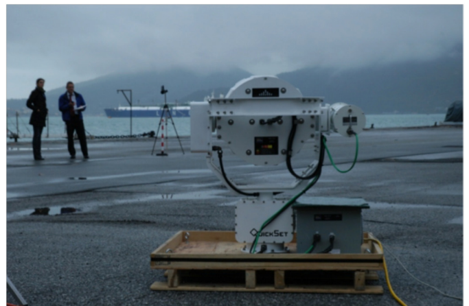
NURC scientists exercise a long-range acoustic device from Ultra Electronics (USA) for use in maritime security operations.
