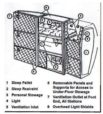
The shuttle orbiter can be outfitted with up to four bunks, three horizontal and one vertical.
