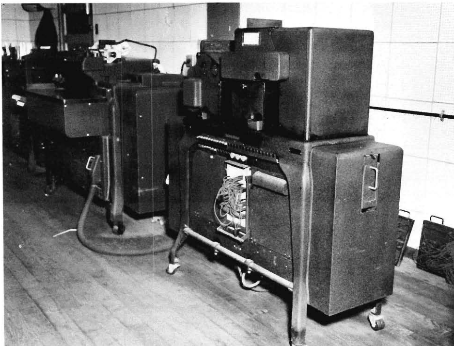
Electromechanical business machines. The lower photograph shows an IBM 513 reproducing punch and, in the background, an IBM 405 alphabetic accounting machine, which could add or subtract and list results with its printer (on top of the machine). The machines were programmed with interchangeable plugboards (upper photograph) that were wired appropriately for the desired calculations or machine operations. A small plugboard is in place on the front of the reproducer and two larger plugboards of the type used in the accounting machine are propped against the wall to the right.
