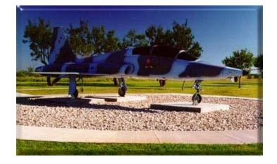
The T-38 was produced for the USAF as its first supersonic jet trainer. The T-38 was used as an advanced trainer for upgrading pilots from the T-37 basic jet trainer to the more maneuverable and faster aircraft they were to later fly. Pilots flying the T-38 gained experience in supersonic flight using its afterburning engines with a top speed of 820 mph.
