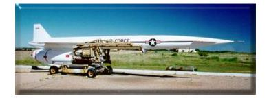
The Hound Dog was designed as a long range, stand-off air-to-ground strategic missile. It was carried in pairs beneath the wings of B-52 aircraft. Its development was initiated by the Air Force in 1957 during the early years of the cold war. It was designed to be carried on airborn alert B-52 aircraft to give them long range strike capability if needed. The first launch took place in 1959 when a Hound Dog was launched from a B-52G.
