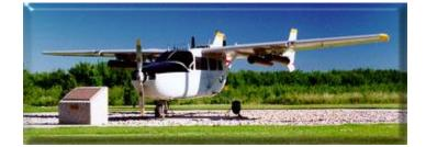
Originally this airplane was a Cessna 337 Super Skymaster. This unorthodox all-metal business aircraft resulted from several years of study by Cessna aimed at producing a twin-engine airplane that would be simple to fly, low in cost, safe and comfortable, while offering all the traditional advantages of two engines.
