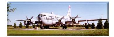
Bill Boeing's company built some very practical airplanes. Fatten the B-29's fuselage, use the same wings, tail and engines and you have a cargo plane. The prototype first flew in 1944 with the first production C-97A in 1949.
