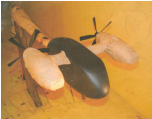
Fig. 16 : Power Model tests: Pusher Configuration
