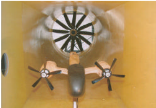
Fig. 15 : Power Model tests: Tractor Configuration
