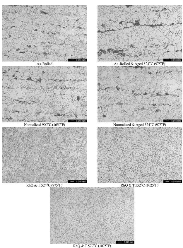
Figure 1. Microstructure of 25.4 mm- (1-inch-) thick plate
