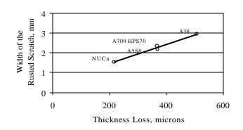
Figure 4. Comparison of the width of the rusted region on the salt sprayed scratched painted steel panels with the thickness loss of the bare steel panels in SAE J2334 tests.
