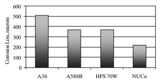
Figure 2. Results of the accelerated corrosion test (automotive SAE J2334 Standard) performed at Bethlehem Steel Company<sup>7</sup>
