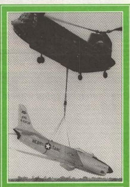
HOW ABOUT A LIFT? - A Kansas Army Reserve CH-47 Chinook helicopter lifts an F-86D Sabre jet restored by the Nebraska Air National Guard to its final resting place in Crete, Neb. Moments after this shot was taken, a retaining strap snapped, requiring an unscheduled landing to re-rig the sling. The Sabre finally did arrive safely in Crete. (Photo by Master Sgt. Lee Straube, Nebraska Air National Guard).
