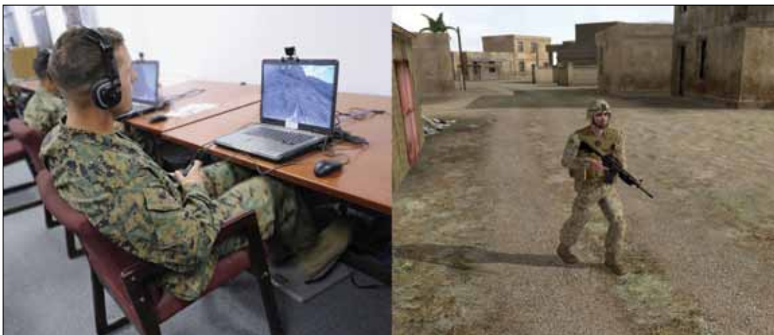
The Pointman avatar controller, developed at NRL's Immersive Simulation Lab, allows users to employ correct tactical infantry movements. Left, Marine operates Pointman via a head tracker, gamepad, and rudder pedals. Right, the user's avatar rendered in Virtual Battlespace 2, a combined arms simulator used by the Marine Corps.
