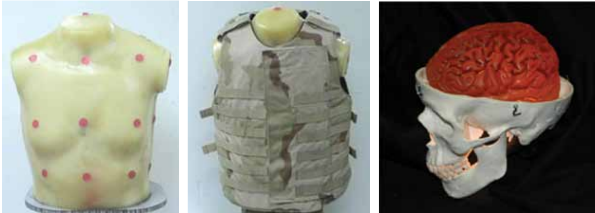
NRL GelMan human surrogate technology is used to record and analyze dynamic responses to blast pressure and impacts. GelMan torso measurement systems assess pressure transmission directly into the body, and through body armor into the body. GelMan-Brain systems quantify headborne protective equipment performance with the aim of reducing traumatic brain injury.
