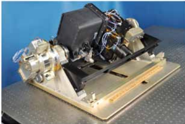
FIGURE 6 The HICO flight imager in the laboratory. The imager is incorporated into a larger payload module that attaches to the Japanese Exposed Facility on the International Space Station.
