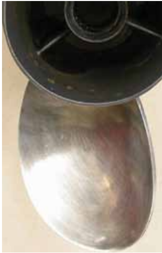
LTIH-316L Prop (15 min) No penetrating damage
