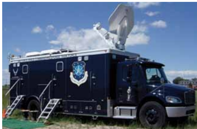
Minuteman InfraLynx Communications System (MICS) – communications trucks designed to support the intercontinental ballistic missile (ICBM) fields in the remote upper midwest.
