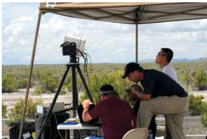
FIGURE 2 Dual Mode Optical Interrogator (DMOI) on tripod.
