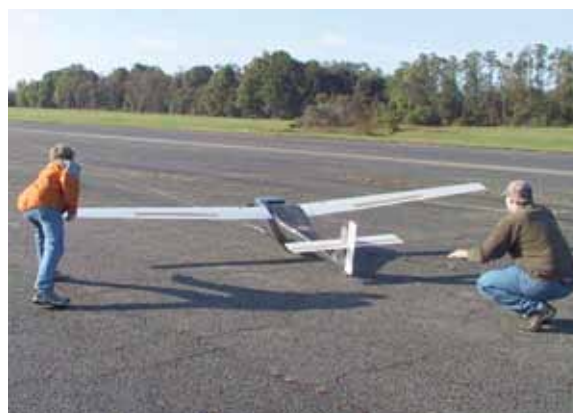
The Ion Tiger being launched for a 23-hr flight at Aberdeen Proving Ground in October 2009.
