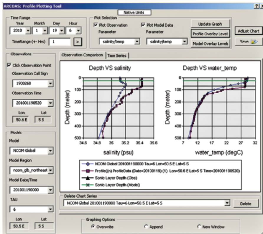
FIGURE 3 Profiles of measured and modeled temperature and salinity plotted from a selected point indicated by the arrow in Fig. 2. The SLD levels overlaid on the profile plots are calculated based on both measured and modeled parameters and show how sensitive SLD is to the ocean thermohaline structure.
