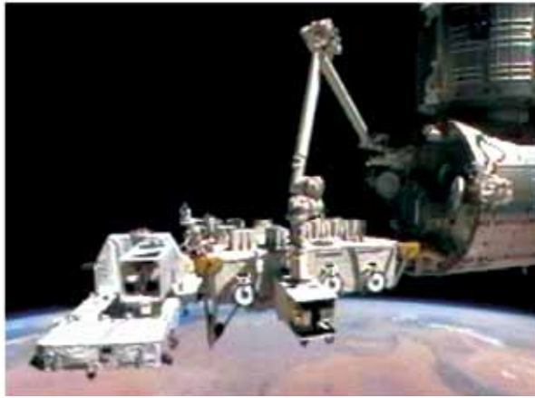
FIGURE 7 The payload module containing HICO is positioned by the Japanese remote manipulator arm prior to attachment to the Exposed Facility (NASA photograph).
