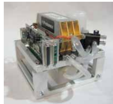
2.2-lb, 550-W polymer fuel cell developed by Protonex Technology Corporation.
