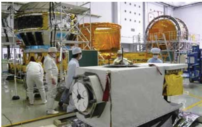
FIGURE 2. HREP (foreground) being prepared for installation aboard JAXA's H-II Transfer Vehicle (background). (Photo: JAXA)
