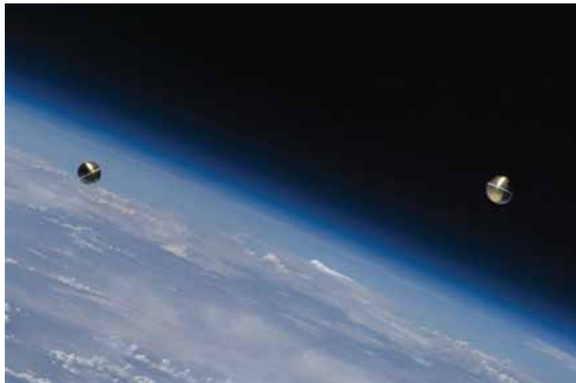
The NRL ANDE-2 twin experimental microsatellites, Castor and Pollux, shortly after deployment under the auspices of the DoD Space Test Program from NASA's Space Shuttle Endeavour (STS-127) on 30JUL09, as photographed by the crew of the STS-127 from the flight deck. ANDE research products are being used to improve methods for the precision orbit determination of space objects, and to calibrate the Space Fence, a radar system of the USAF 20th Space Control Squadron that tracks low-Earth-orbiting space objects.
