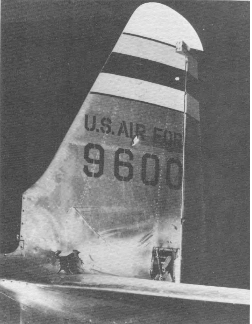
Battle damage to the tail assembly of an F-80.
