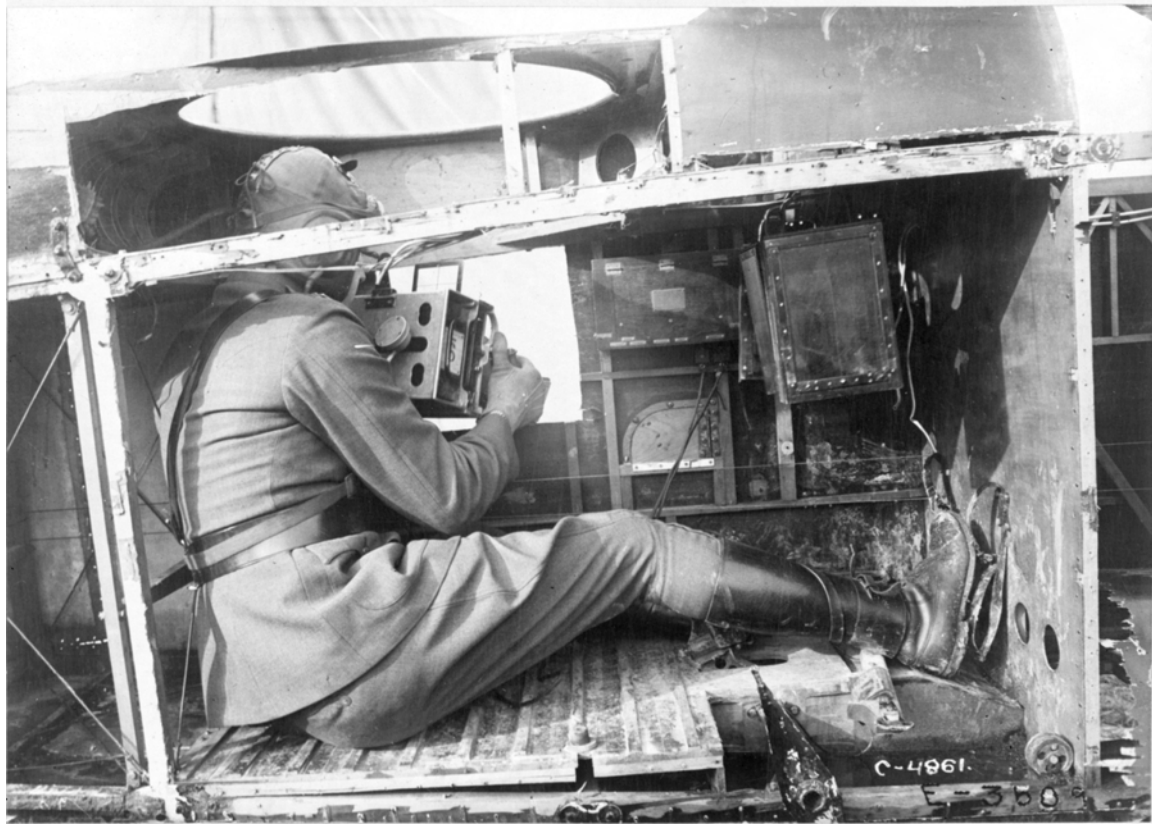
Figure 7. 2 nd A.I.C. Aerial Photography School, Tours. Demonstration of aerial photographer's technique for oblique photography, using a cut-away segment of the De Havilland DH-4 fuselage. It appears that the photographer is wearing a chest-mounted microphone for communication with the pilot. U.S. National Archives and Records Administration, Still Pictures, E-6402.
