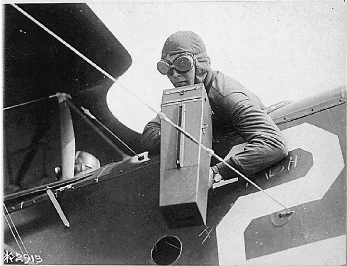
Figure 3. Hand-held Aeroplane Graflex Camera, circa 1917 to 1918. This photograph depicts many of the conditions mentioned in the text, including the rudimentary sighting device, exposed position of the observer, the difficulty of communication between the observer and the pilot, and the obstacles presented by struts and wires. U.S. National Archives and Records Administration, Still Pictures, ARC 530712.
