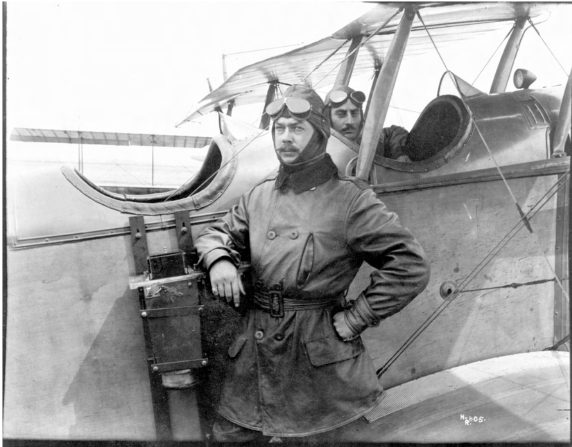
Figure 4. Curtiss JN-4, with external mount for aerial camera. The camera appears to be a (British) Thornton-Pickard "Type C" (or variant thereof) first manufactured in 1915. U.S. National Archives and Records Administration, Still Pictures, E-6401.
