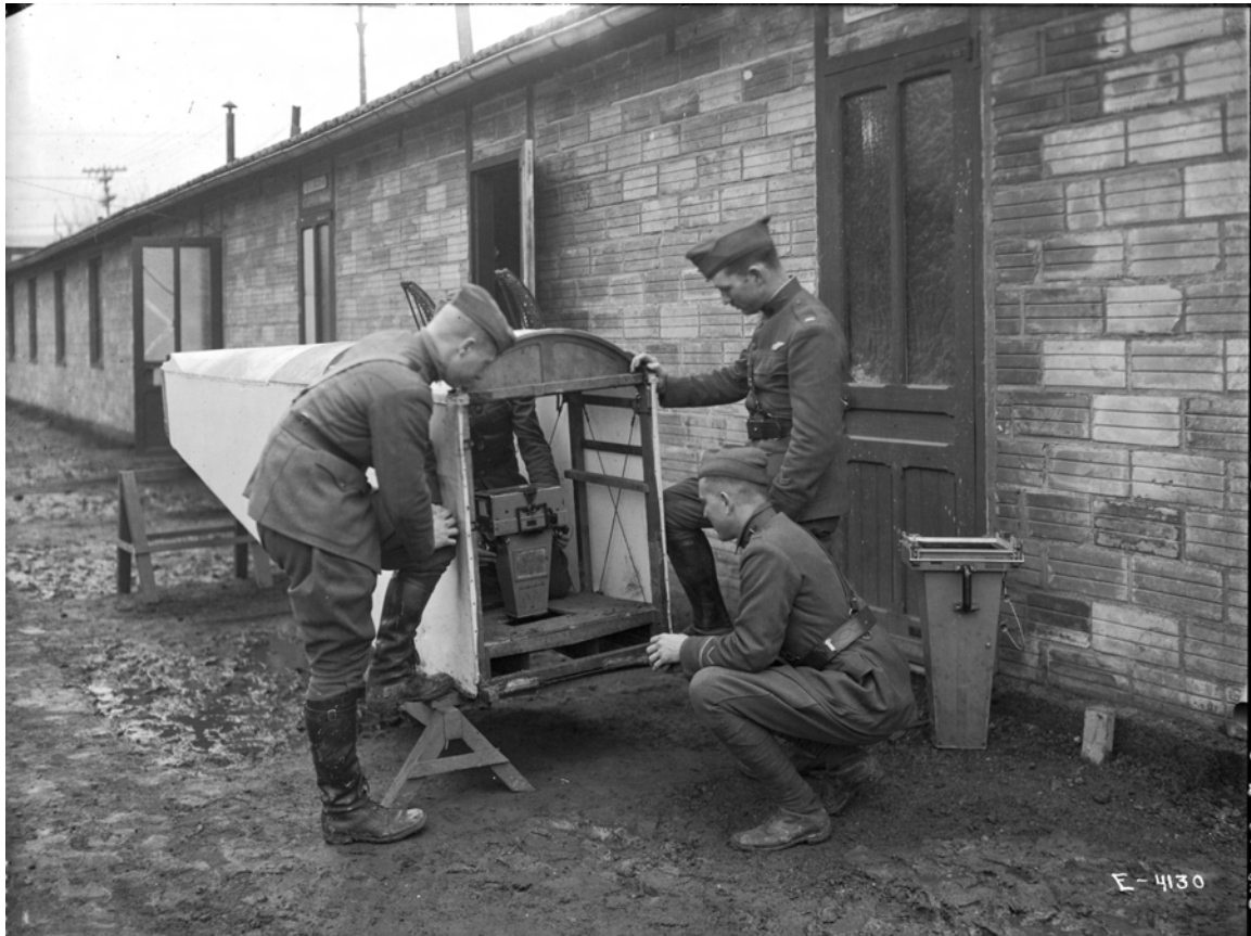
Figure 8. 2 nd A.I.C. Aerial Photography School, Tours. Students examining a cutaway fuselage demonstrating mounting of aerial cameras oriented for vertical photography. U.S. National Archives and Records Administration, Still Pictures, E-4130.
