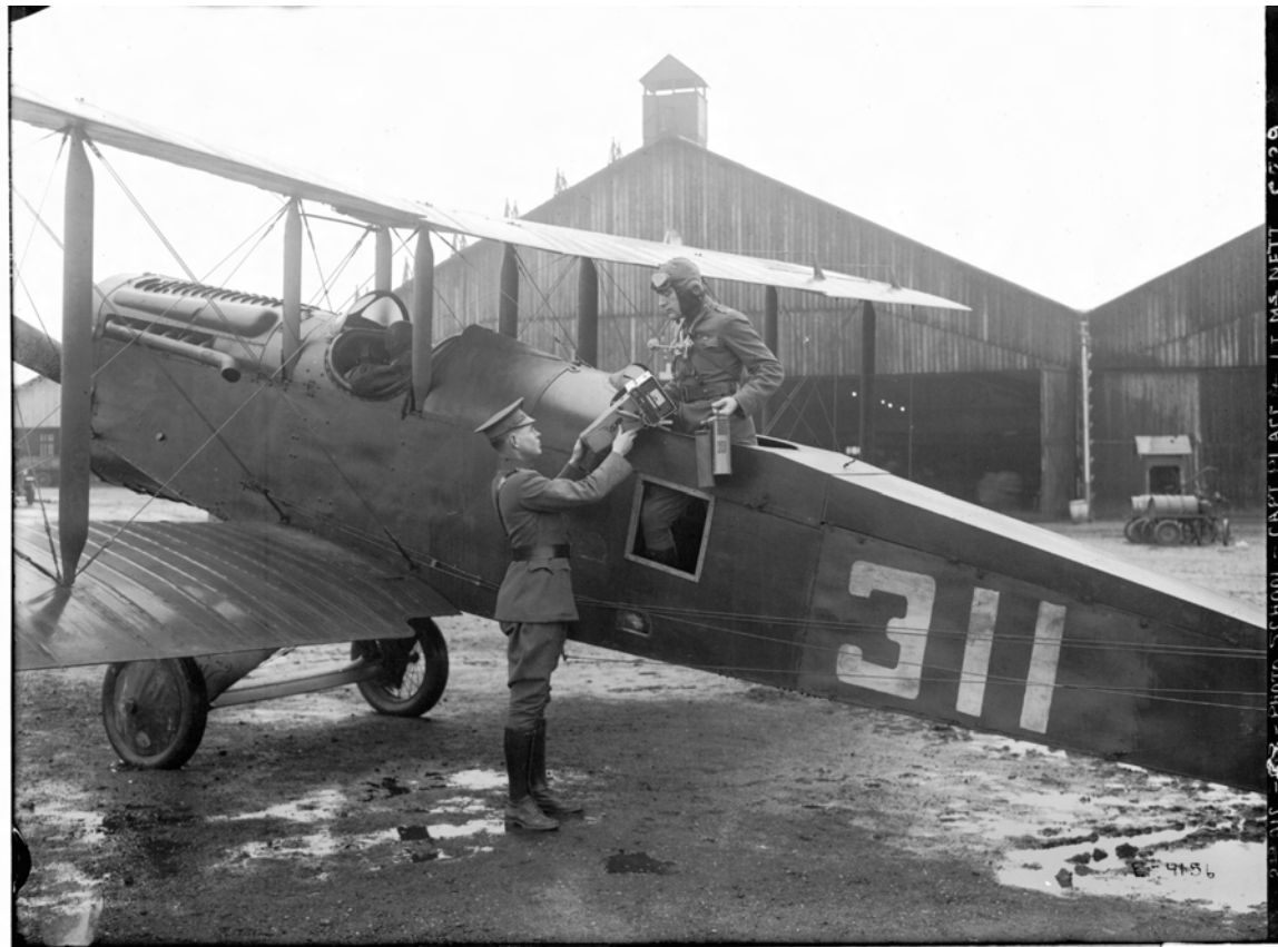
Figure 5. De Havilland DH-4, with port for oblique photography. The photographer wears a chest-mounted microphone for communication with the pilot, and holds a supply of plates for the camera. U.S. National Archives and Records Administration, Still Pictures, E-4156.
