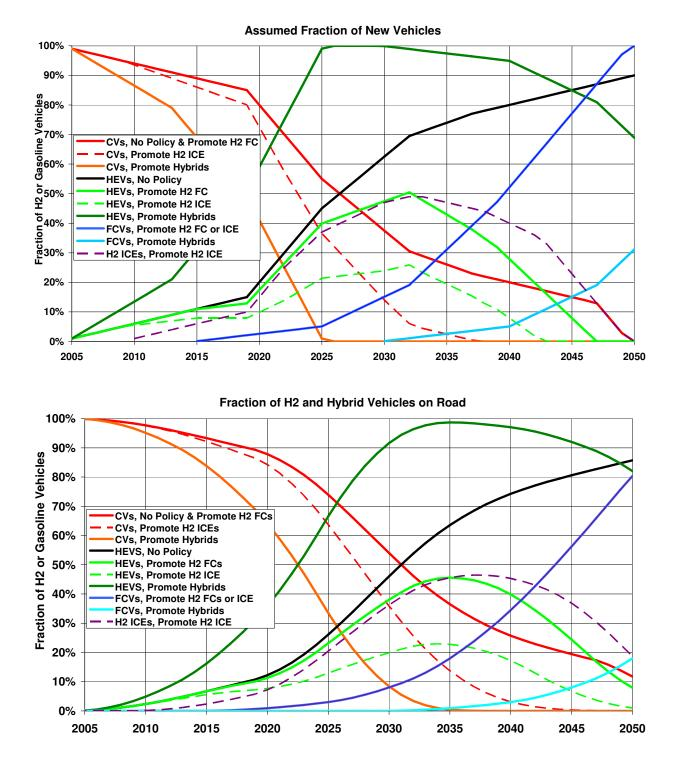
Figure 3. Scenarios of Vehicle Adoption. Top: New Vehicles; Bottom: Vehicle Fleet.
