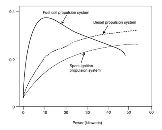
Figure 2. Comparisons of power train efficiency of combustion engine and fuel cell systems (for a car similar to a Volkwagen Golf).
