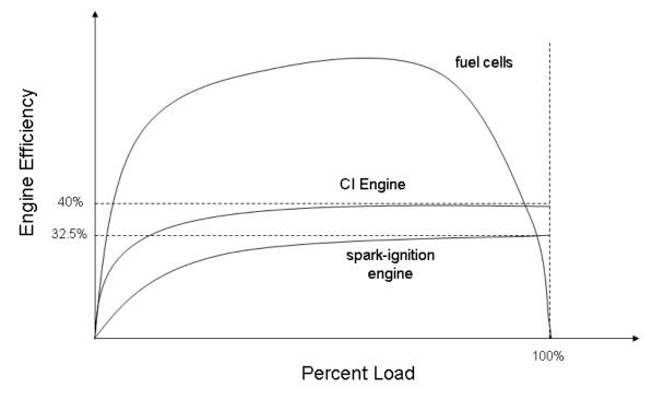
Figure 1. Engine Efficiency versus Load for Fuel Cells, Compression-ignition, and Spark-ignition Engines
