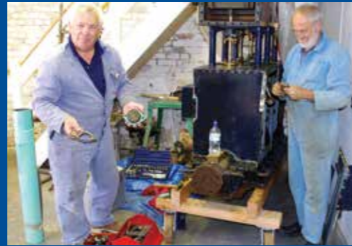
Frank Fowler and Philip Atkinson working on 199's two cylinder compound engine built by Mumford of Colchester around 1920. Frank was demonstrating the ancient art of steam joint making using a hammer.
