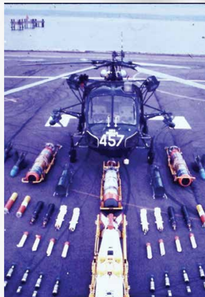
Wasp helicopter weapon load showing a WE 177A tactical nuclear depth bomb in the foreground (Explosion! Museum)
