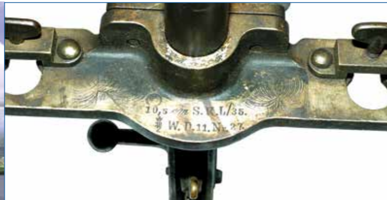
Markings on the bushing piece of the JB 71 rifle, which was used as a basis for the device. The new trigger box was attached to the two screws on the underside.
