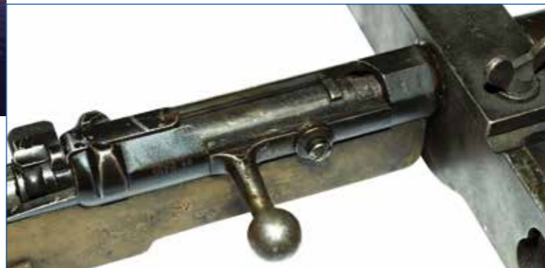
Markings on the bushing piece of the JB 71 rifle, which was used as a basis for the device. The new trigger box was attached to the two screws on the underside.
