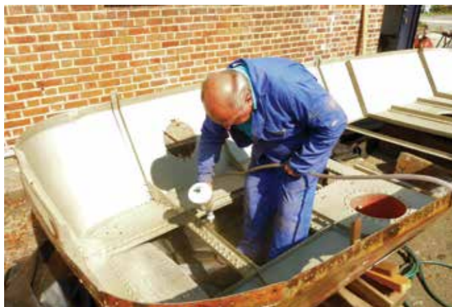
Alistair Dilley spray painting the inside of the machinery space cover.
