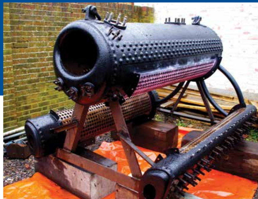
The boiler has been returned with its tubes removed, mounted in a frame to retain the steam drum/water drums relative positions. Weld repair work on the drums has been non-destructive tested and approved by the boiler examiner.
