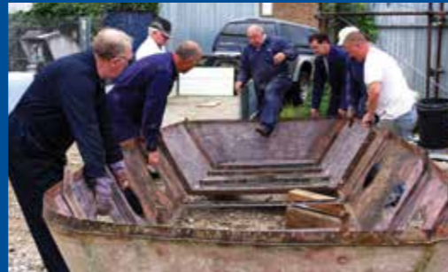
Moving the machinery space canopy after removing all the paint – it is upside down.
