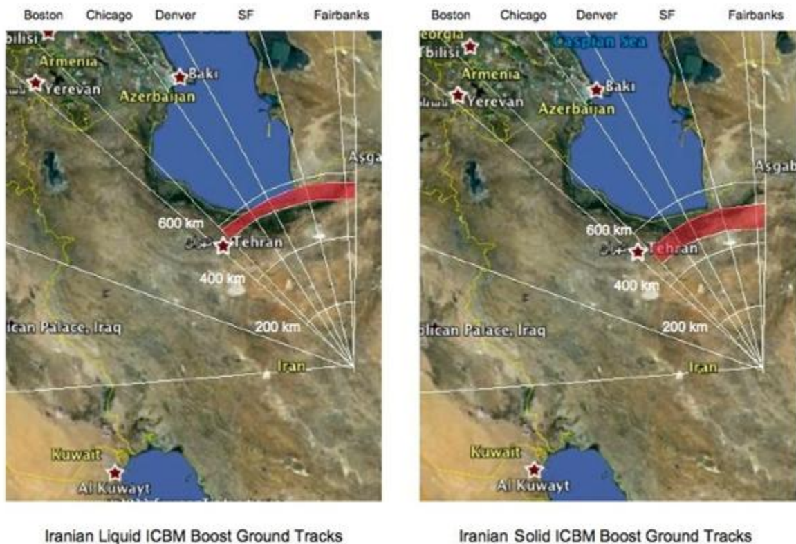
FIGURE 2-14 Fly-out ground tracks and azimuths for notional liquid and solid ICBMs launched toward North America from central Iran.
