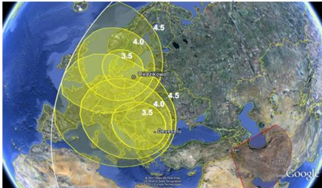
FIGURE 3-7 Notional SLS footprints against minimum energy trajectories from Iran for interceptors with fly-out velocity varied parametrically between 3.0 and 4.5 km/sec based at Deveselu, Romania, and Redzikowo, Poland. EOR is assumed.
