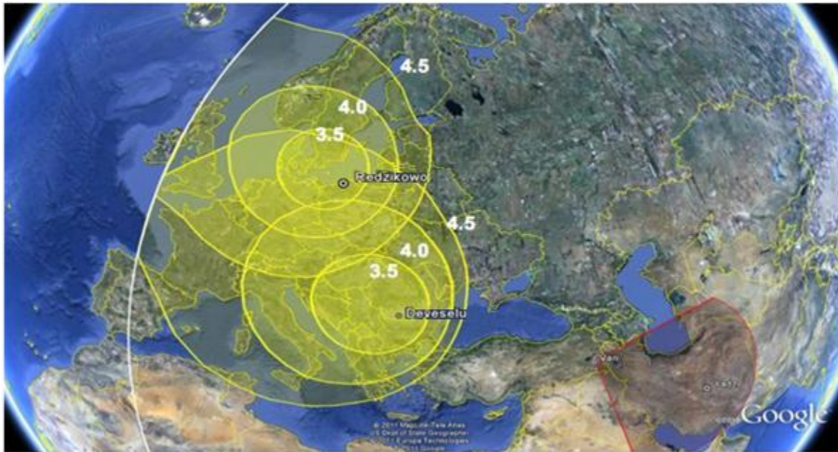
FIGURE 3-8 Notional SLS footprints against lofted trajectories from Iran for interceptors with fly-out velocity varied parametrically between 3.0 and 4.5 km/sec based at Deveselu, Romania, and Predzikowo, Poland. EOR is assumed.
