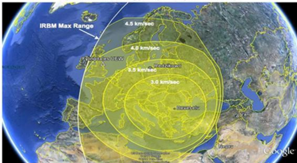
FIGURE 3-4 Notional single-shot coverage for interceptors with fly-out velocity varied parametrically between 3.0 and 4.5 km/sec against minimum energy notional 5,600-km solid IRBM trajectories from central Iran. EOR is assumed.
