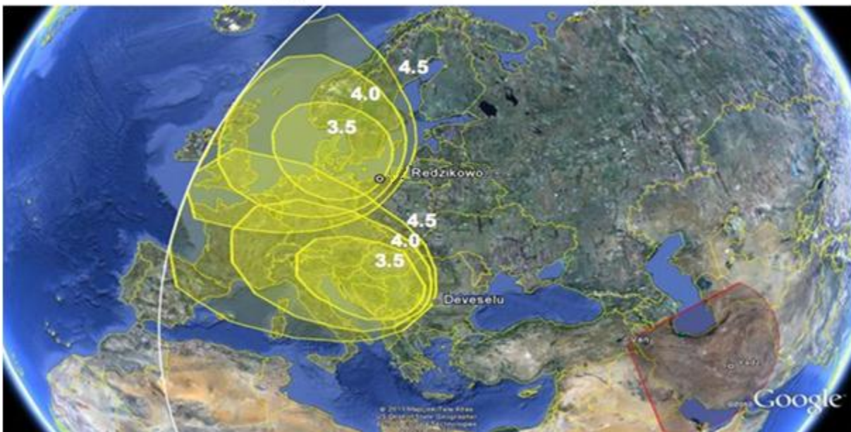
FIGURE 3-9 Notional SLS footprints against depressed trajectories from Iran for interceptors with fly-out velocity varied parametrically between 3.0 and 4.5 km/sec based at Deveselu, Romania, and Redzikowo, Poland. EOR is assumed.
