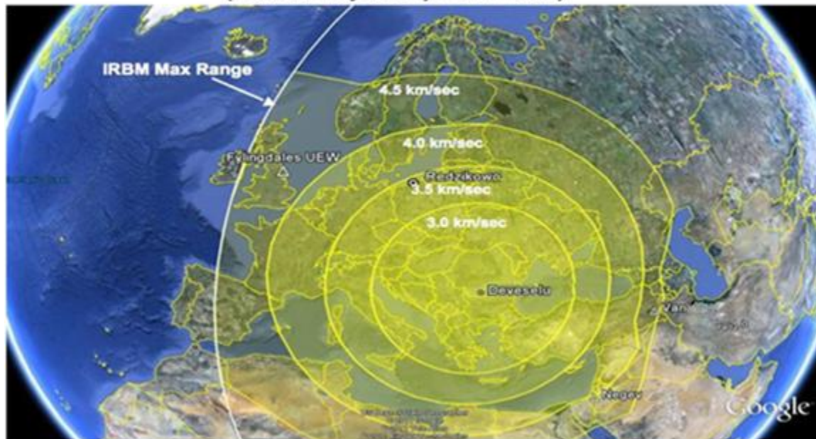
FIGURE 3-5 Notional single-shot coverage for interceptors with fly-out velocity varied parametrically between 3.0 km/sec to 4.5 km/sec against lofted trajectories from central Iran. EOR is assumed.
