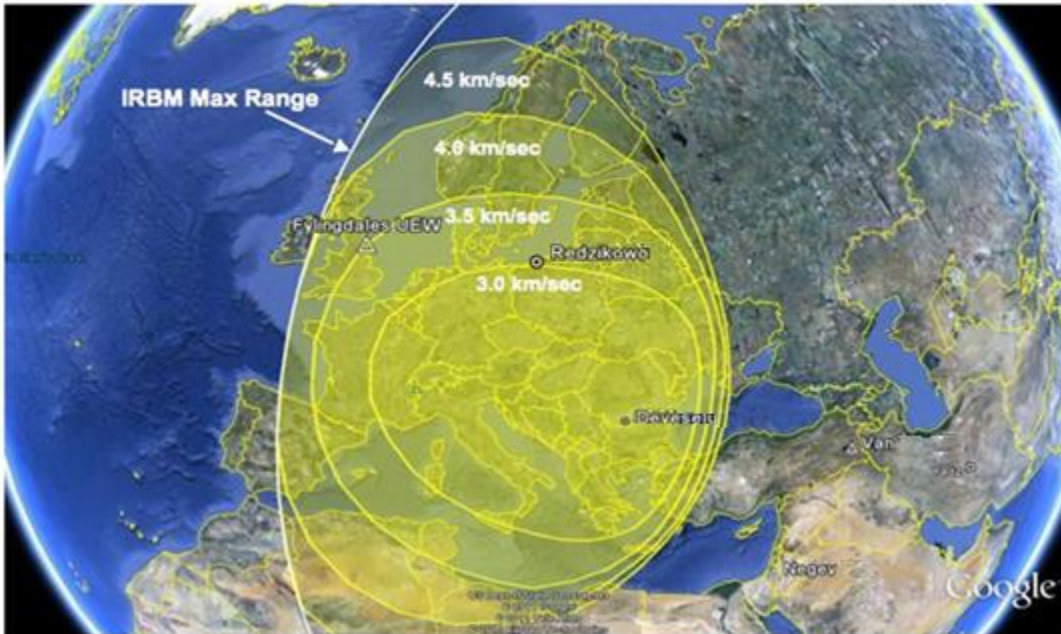
FIGURE 3-6 Notional single-shot coverage for interceptors with fly-out velocity varied parametrically between 3.0 and 4.5 km/sec against depressed trajectories from central Iran. EOR is assumed.
