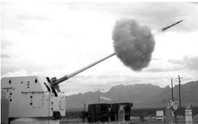
The projectile is captured just as it leaves the 5-inch gun at LC-35 in this high-speed photo. Photo from the Jerry Crouch Collection.
