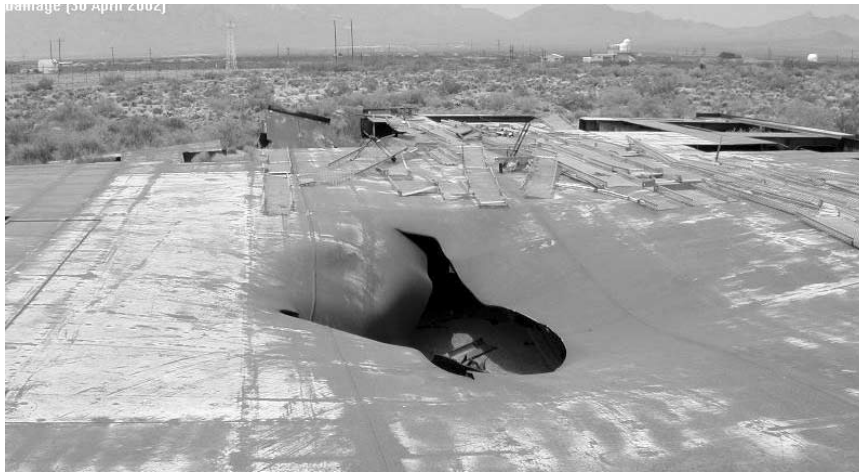
The gaping hole in the simulated ship decking, just north of the Navy blockhouse at LC-35, was a result of Operation Pushover No. 2
