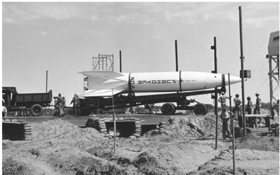
The V-2 rocket used for Operation Pushover No. 2 in 1949 sits ready to be erected on the simulated ship deck just north of the Navy blockhouse at LC-35.
