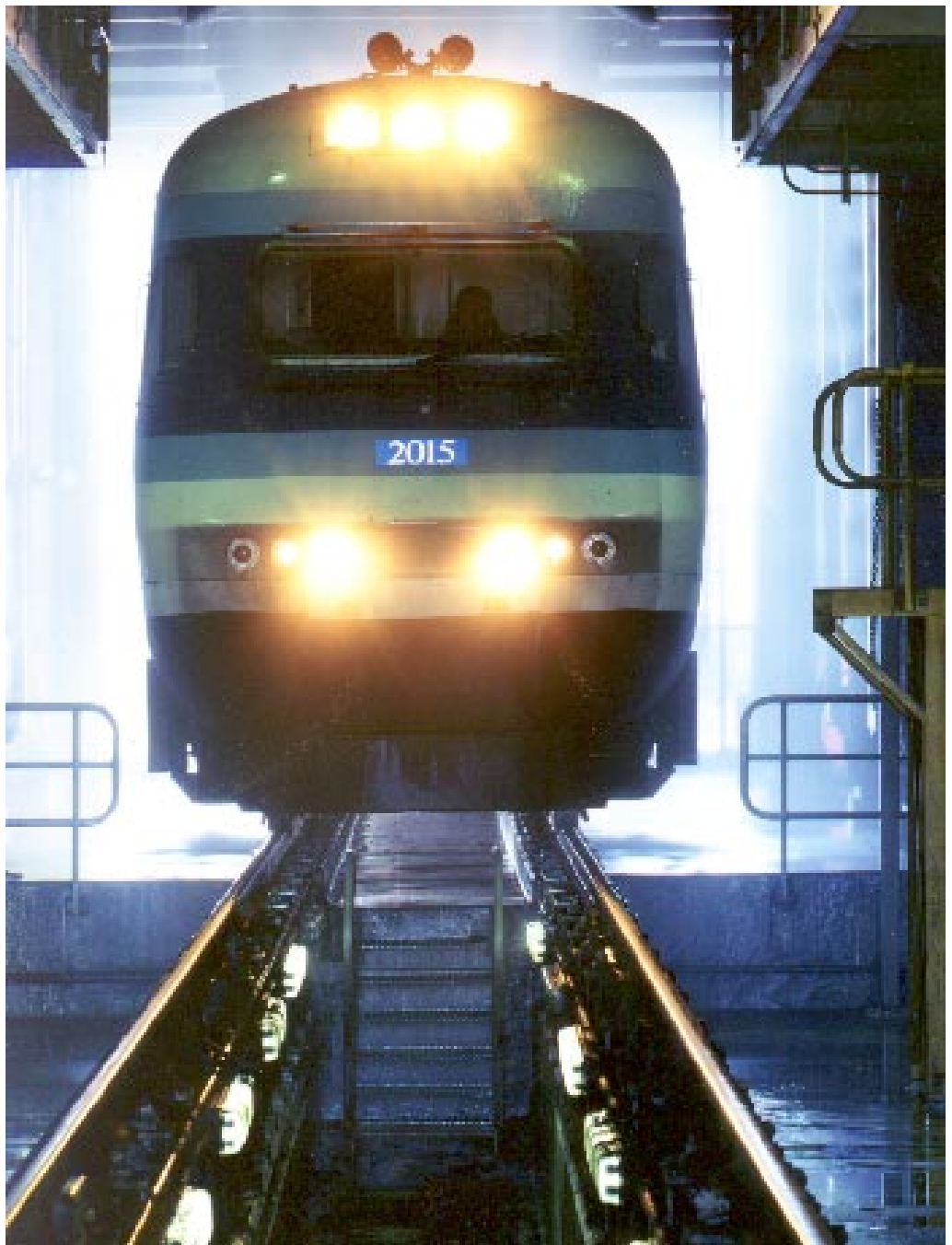
An Intercity XPT goes through the wash plant at Sydenham's XPT Service Centre
