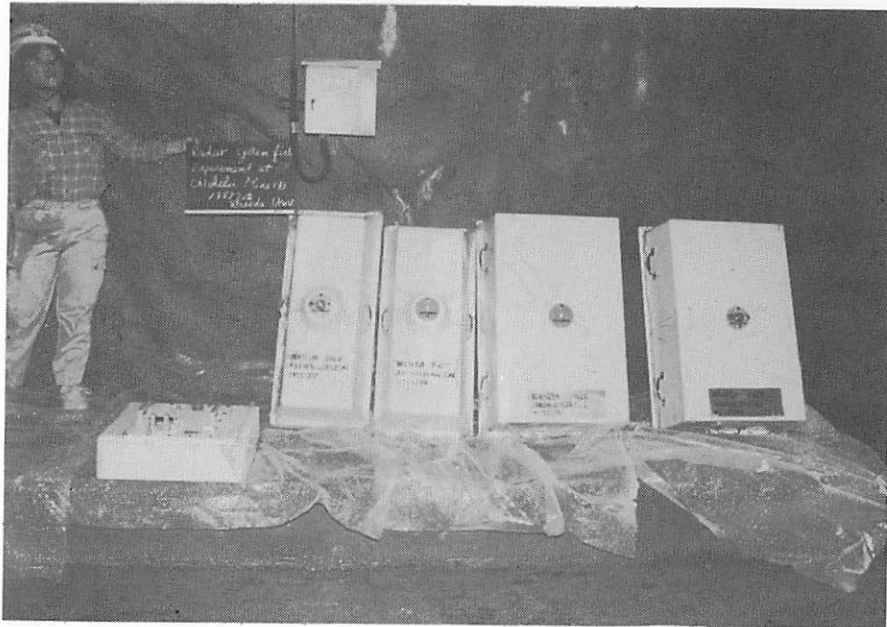
Fig. 9 Antennas used for this survey (400MHz, 150MHz, 80MHz)
