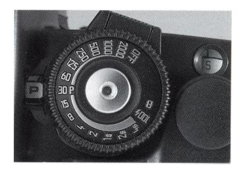
When using non-system flash units, the shutter speed must be set to "100". In the "B" setting, the shutter remains open for a long as the exposure release button is pressed down. The symbol "bulb" is displayed in the viewfinder.
