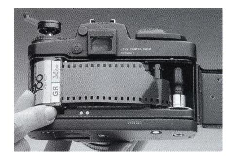
Pull up the rewind crank as far as it will go and insert the film cartridge in the empty cartridge chamber, then push in the rewind crank. The edge of the film must be parallel with the film guide. As you move the quick-wind lever, the sprockets of the transport drum must engage in the edge perforations of the film.
