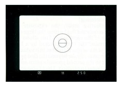
The camera automatically computes the shutter speed from 1/2000 s and 16 s, depending on the available light. The shutter speed setting dial may be set to any shutter speed from 1/2000 s to 4s, except "B", or "100".
