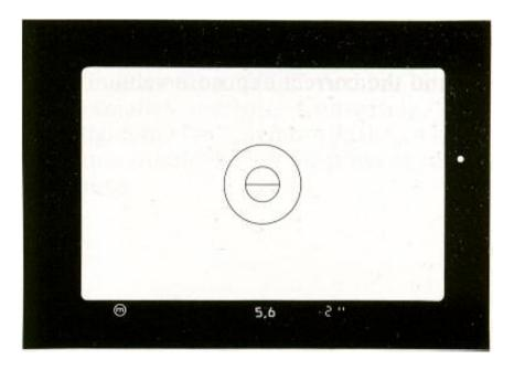
P lights up. For deviations in the -1.5 to +1.5 range, this can be read in ½ Ev. Aperture or shutter speed must be adjusted until the symbol ● - i.e. correct exposure-lights up.
