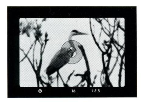
The remainder of the screen looks like a groundglass screen and is ideal for focusing telephoto lenses and for close-range photography.
