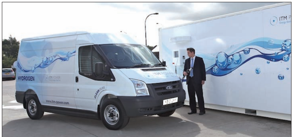
ITM Power's HFuel ® system for refuelling hydrogen-powered vehicles is based around a modular platform (packaged in a standard freight container), and can be expanded at any time to allow a staged rollout of hydrogen fuelling infrastructure.
