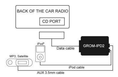
Figure 3. Basic wiring diagram.
