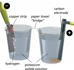
Electrolysis of potassium iodide solution. In the photo below, a porous diaphragm separated the cathode and anode compartments. This does not prevent the current from passing through — just as a paper bridge does not.
