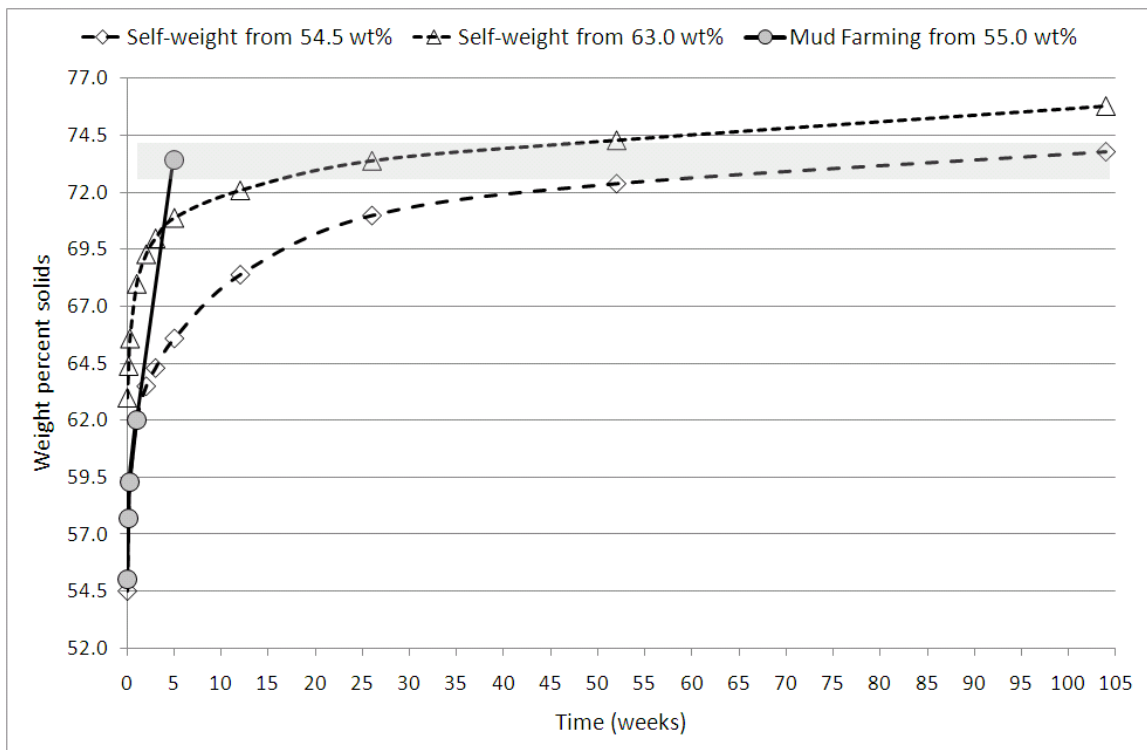
Figure 5 Effect of an enhanced AST consolidation regime on residue consolidation rate versus natural consolidation rates. Shaded area between 72.5 and 74.0 wt% solids indicates target solids content for continued construction.
