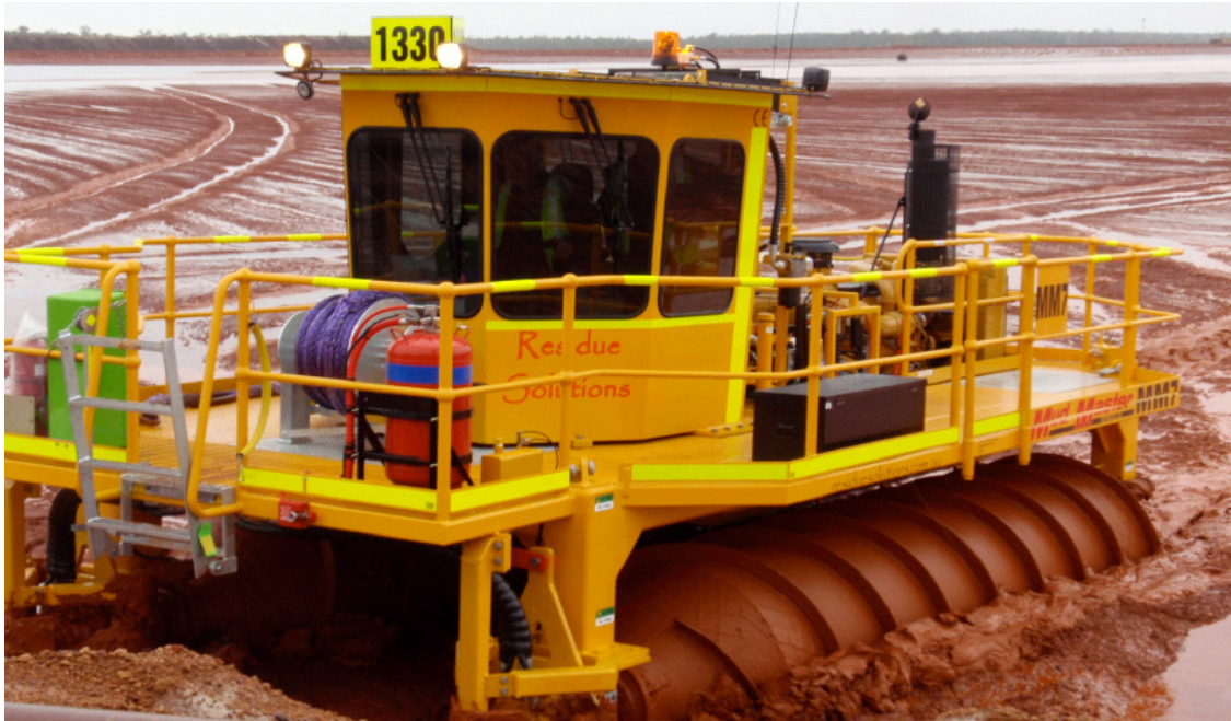
Figure 2 An AST being commissioned in fresh bauxite residue.
