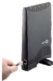
Figure VII.2: Pre WiMAX: Indoor Customer Premises Equipment (CPE) containing an antenna, transceiver and modem.
