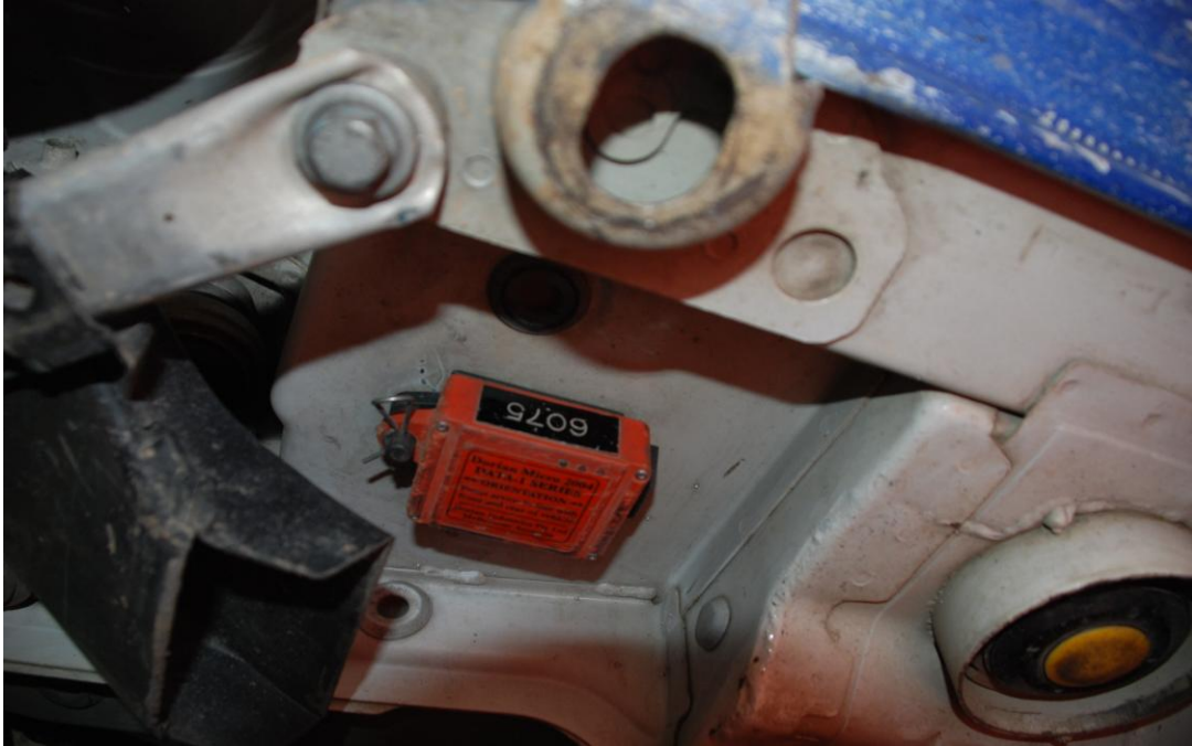
LOCATION OF DORIAN DATA 1 MICRO TIMING TRANSMITTER (FLOOR PAN REMOVED)
